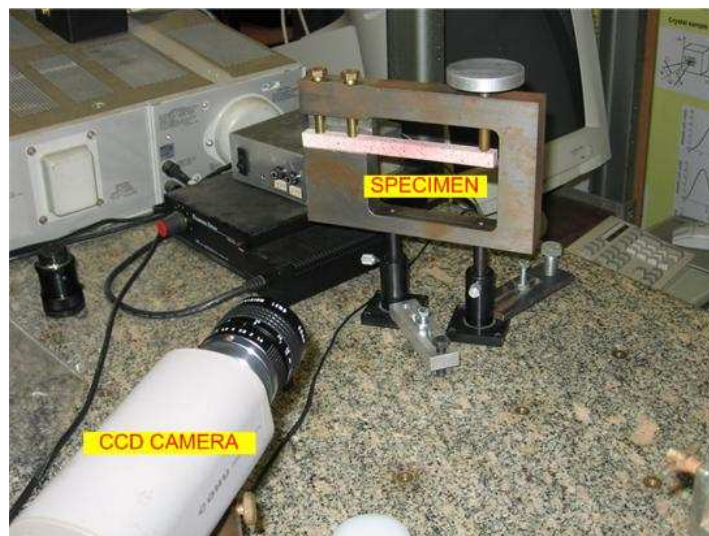
Figure 3: Experimental arrangement of DIC method.
