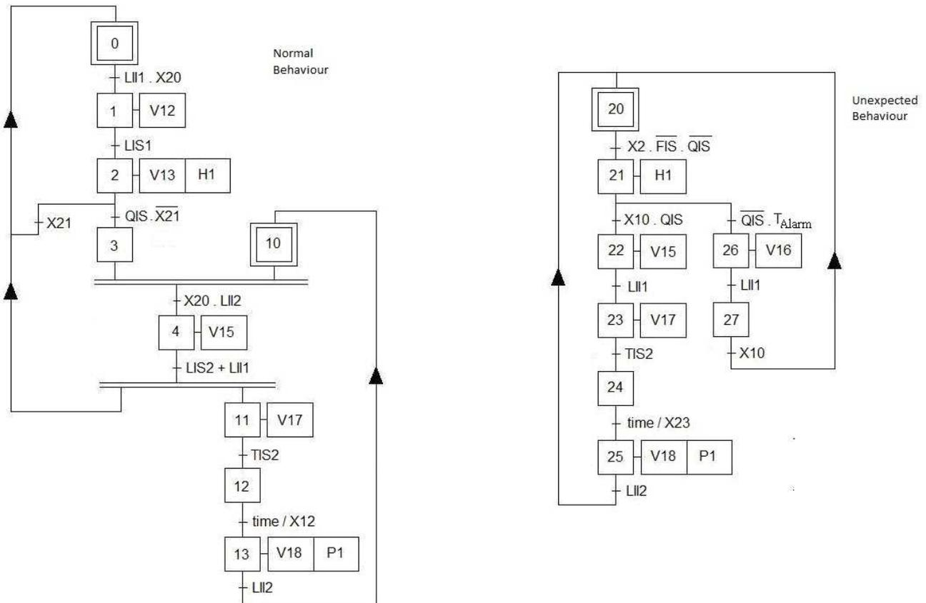
Figure 3. SFC controller specification: normal and unexpected behavior modes.
