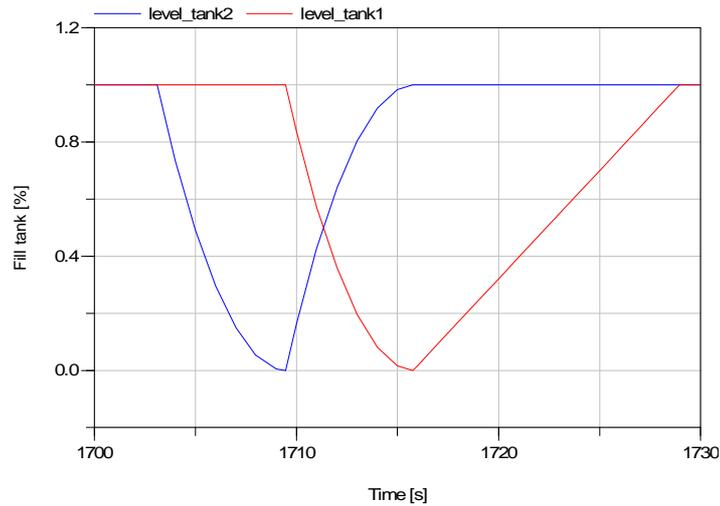
Figure 8. Level tanks in function of time with a heat supply rate of 3170W for the solution transfer time period between tank1 and tank2.
