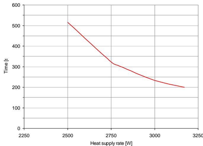
Figure 9. Time for the solution powder-processing operation fulfilled in the tank2 in function of heat supply rate.
