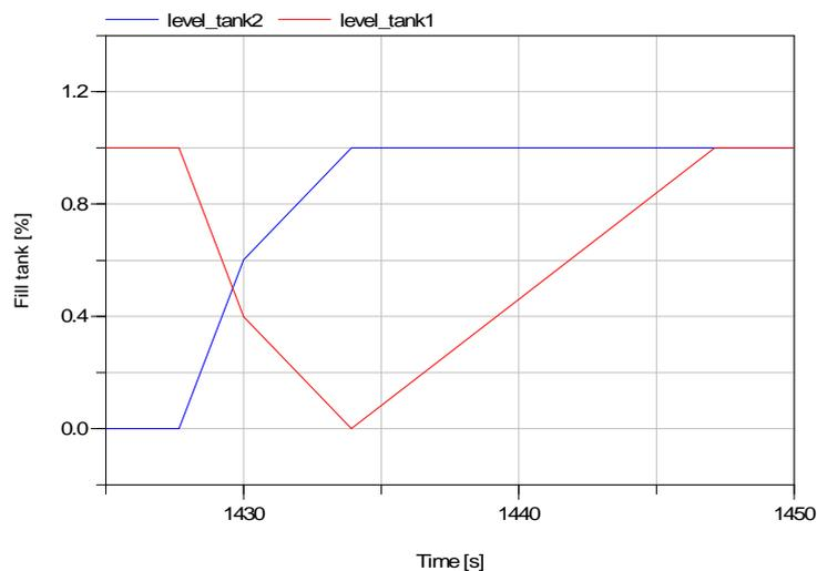
Figure 5. Level of tanks in function of time in normal operation of the evaporator system.
