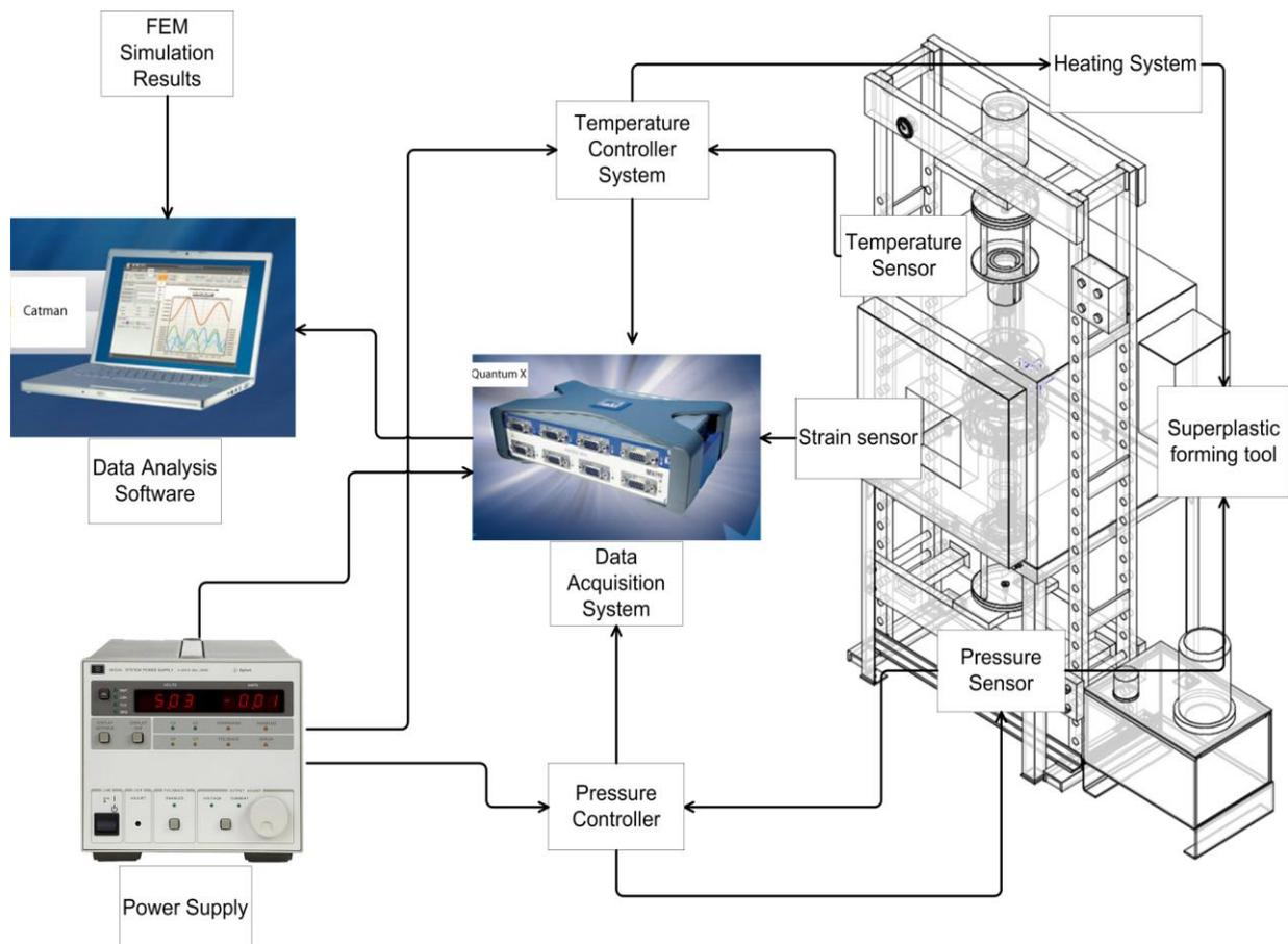
Fig. 7 Experimental Setup (Marinho et al., 2011)
