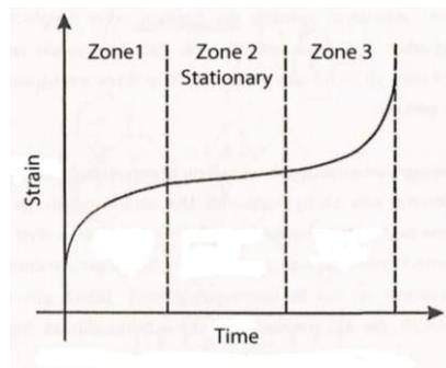
Fig. 6 - Sigmoidal curve - Strain vs. Time (Samekto, 2005)
