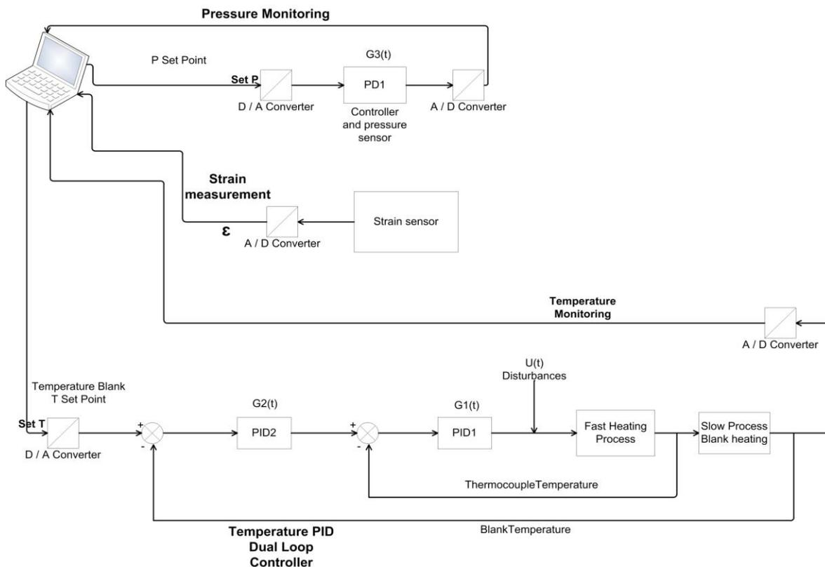
Fig. 10- Independent Control System (Temperature, Pressure and Strain) (Marinho et al., 2011)
