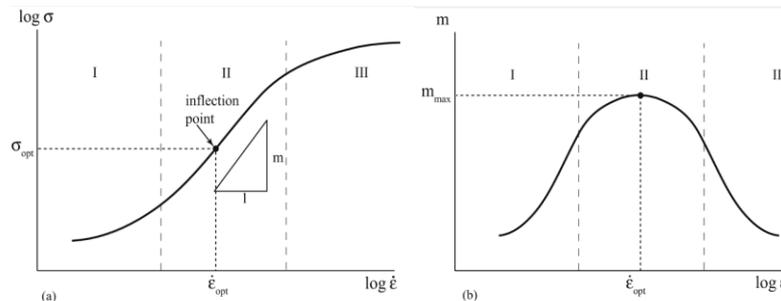
Fig. 9 - Typical behaviour of superplastic materials: (a) Curve showing the sigmoidal behaviour of the flow stress logarithm versus strain rate logarithm. (B) the strain rate sensitivity "m" versus strain rate logarithm (Snippe Q.H.C.,2009)
