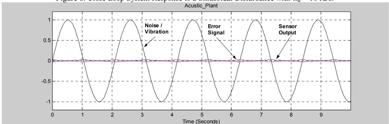
Figure 9. Close Loop System Response to a Sinusoidal Disturbance with  $\omega_d = 3$  rd/s.
