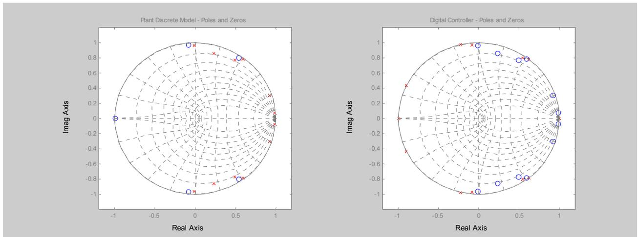
Figure 6. Plant and Controller Poles and Zeros.
