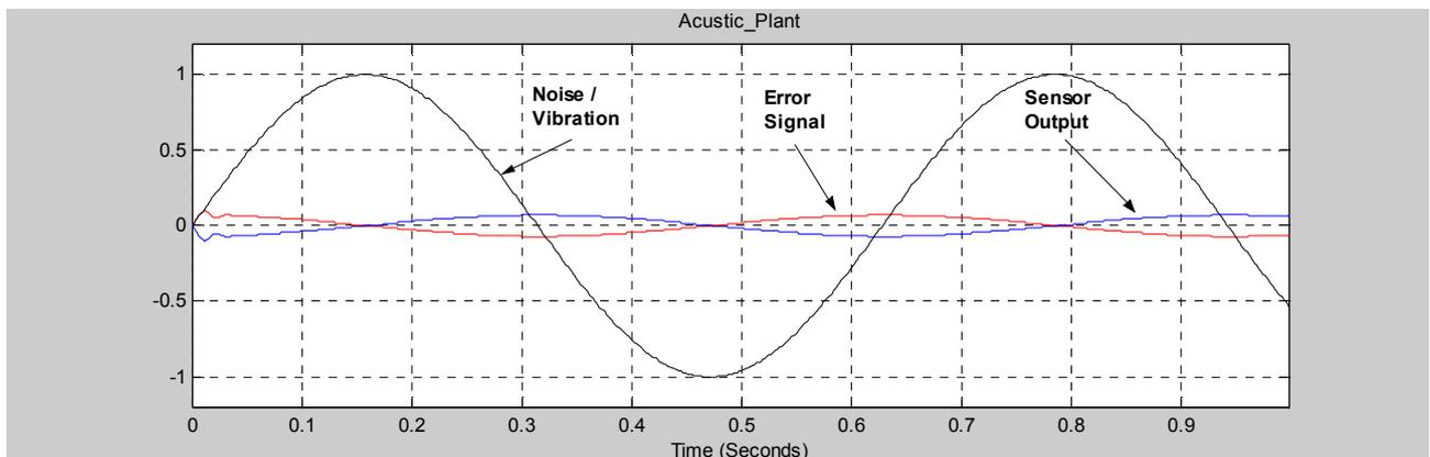
Figure 8. Close Loop System Response to a Sinusoidal Disturbance with  $\omega_d = 10$  rd/s.
