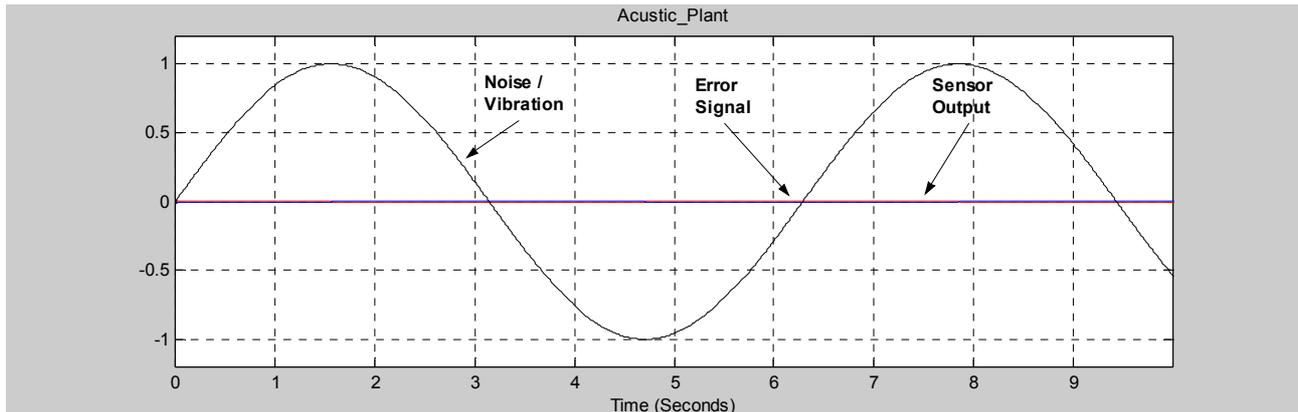
Figure 10. Close Loop System Response to a Sinusoidal Disturbance with  $\omega_d = 1$  rd/s (the best case).
