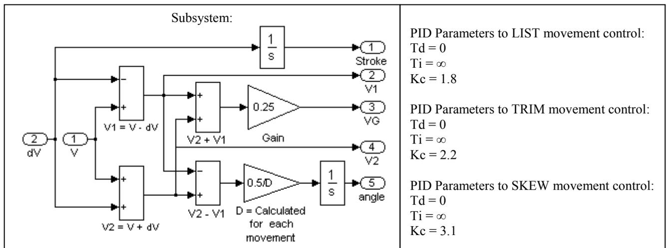
Figure 8. Closed loop control to TRIM, LIST e SKEW movements
