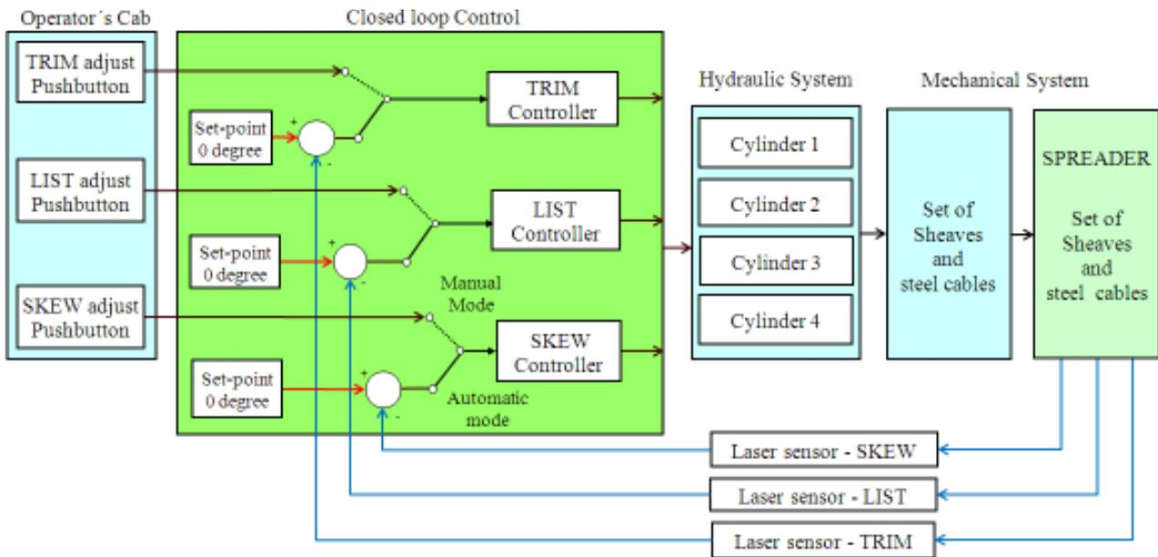
Figure 4. Block diagram of the proposal system to control the spreader
