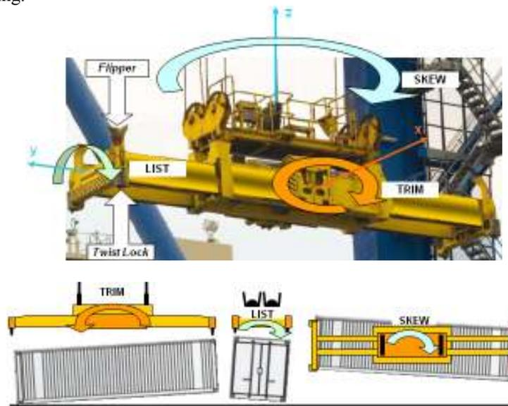
Figure 2. Spreader movements
