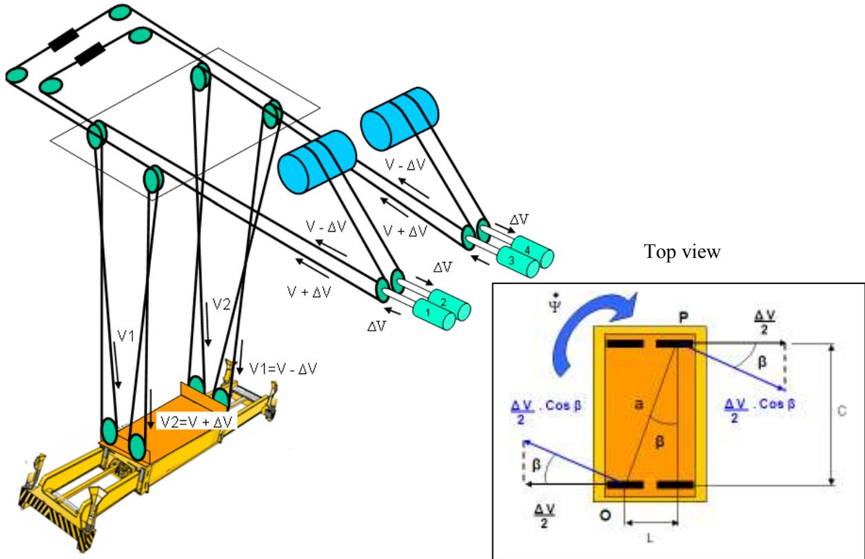
Figure 7. Composition of the angular velocity of SKEW movement
