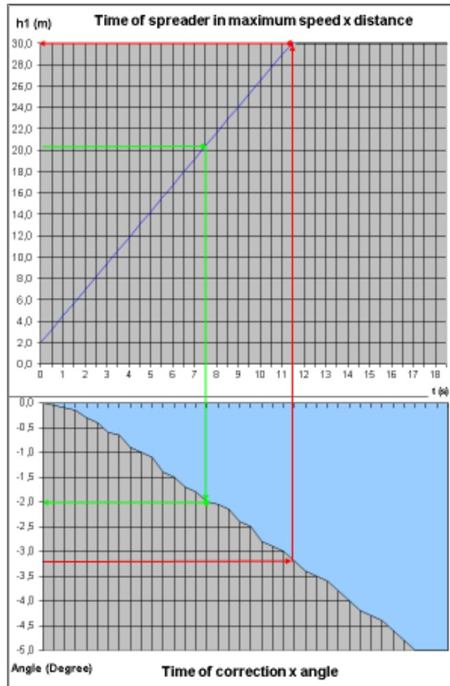
Figure 11. Correlation of the travel of the spreader and the angle corrected in the SKEW movement
