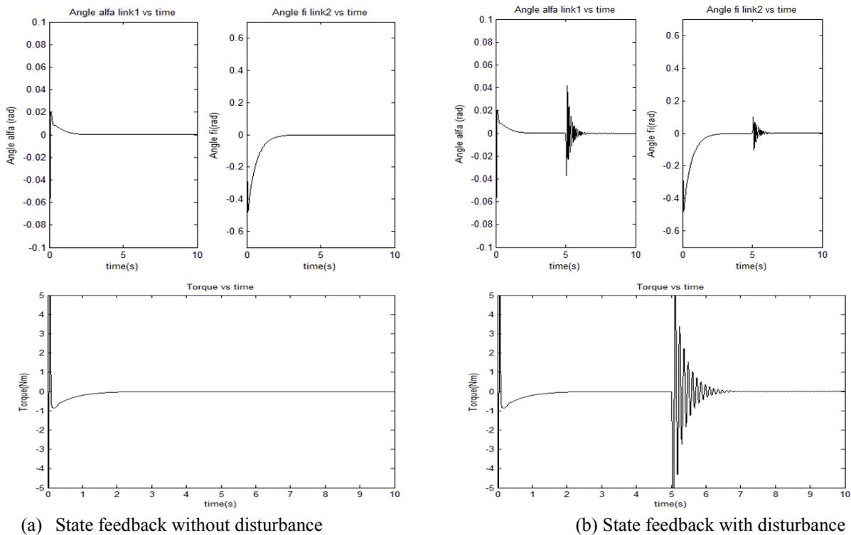
Figure 5. System controlled by state feedback.
