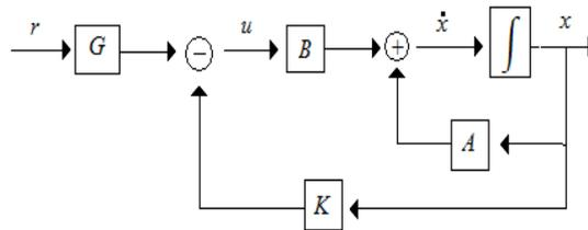
Figure 3. The block diagram of the state-feedback controller.
