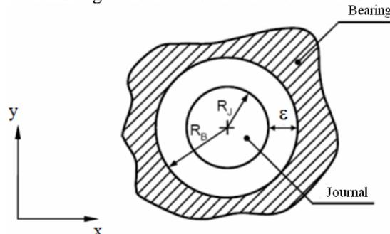
Figure 1. Revolute joint with clearance.
