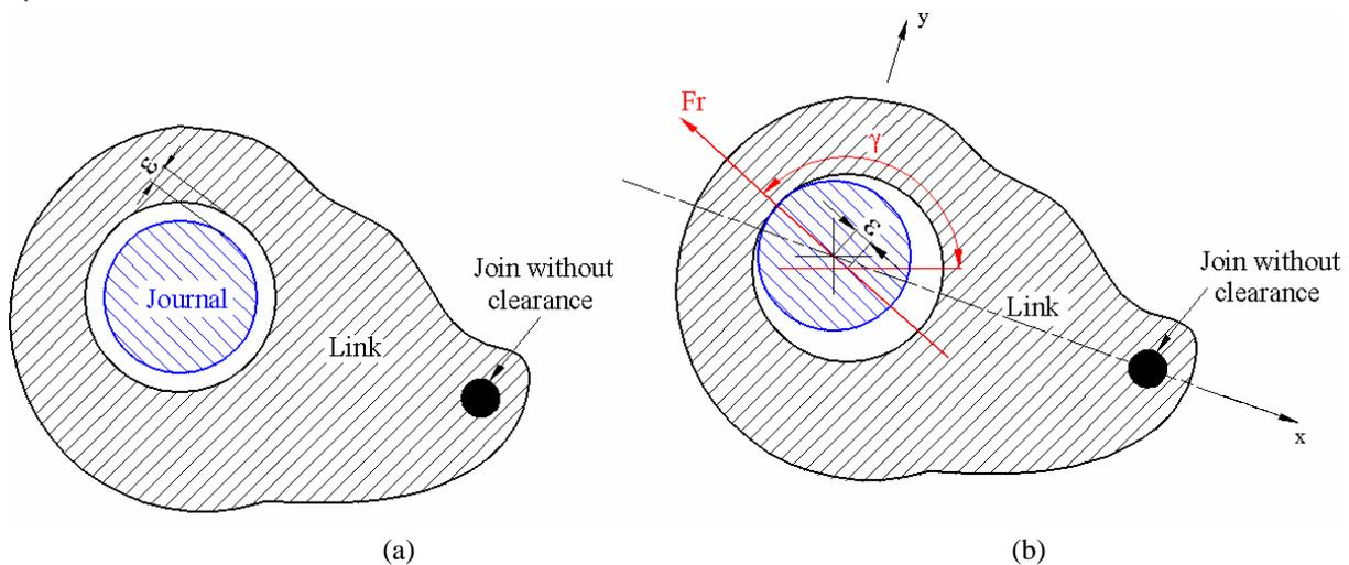
Figure 3. (a) Model of clearance; (b) Reaction force.
