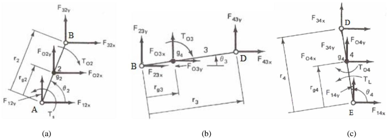
Figure 5. (a), (b) and (c) show free-body diagrams of links used for the kinetostatic equilibrium (Erdman and Sandor, 1991).
