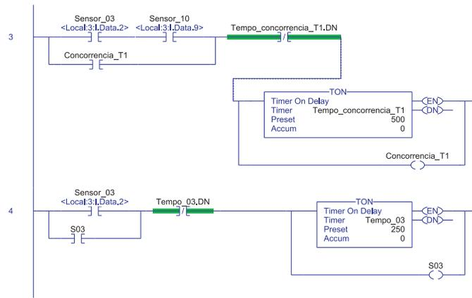
Figure 6. Block  $Tv_3$  energizing concurrency treatment in *ladder*
