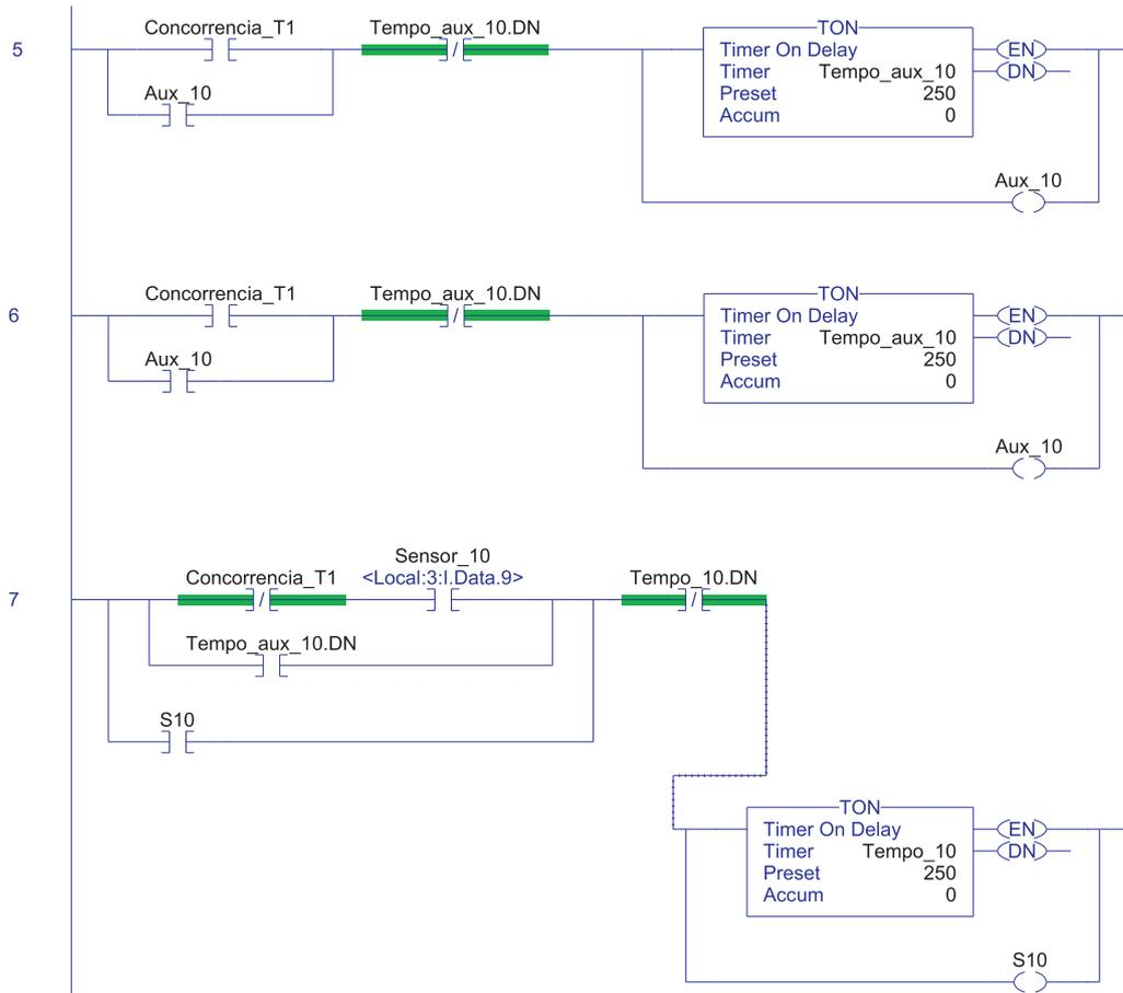
Figure 7. Block  $T_{v3}$  energizing concurrency treatment in ladder
