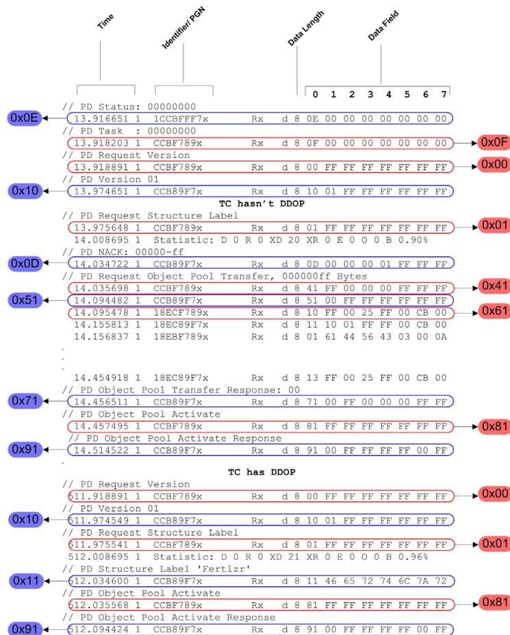
Figure 7. The CAN messages log of the initialization process among ECU1 and ECU4.
