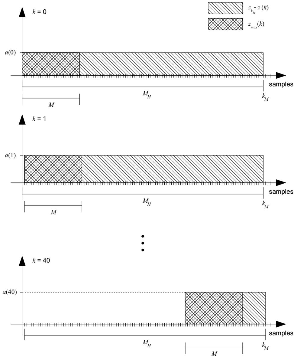
Figure 2. Evolution at time of the amount of accumulated degradation  $Na(k)$  that can be spent during a predict window.
