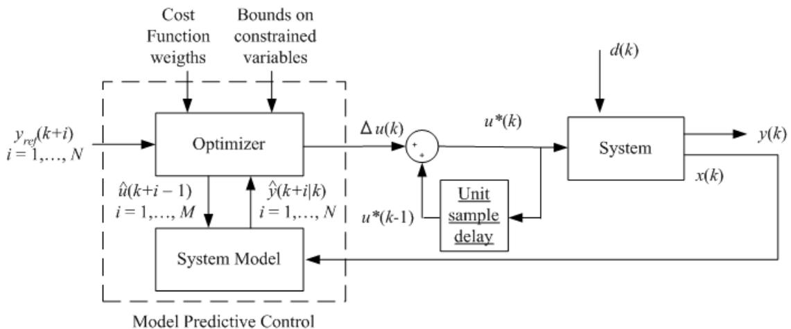
Figure 1. MPC scheme employing state feedback.
