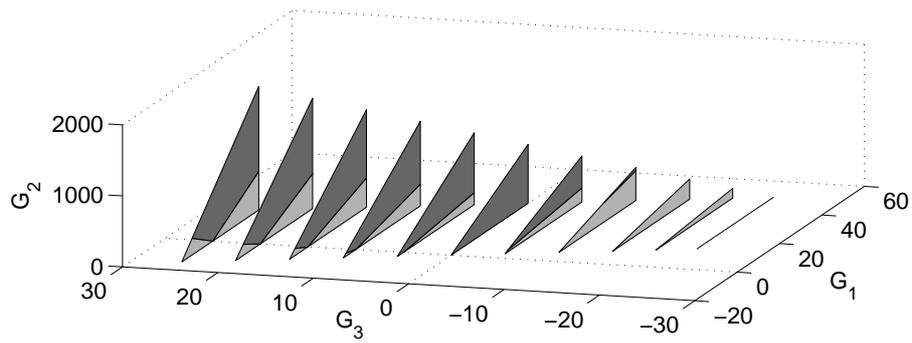
Figure 7. Lead/lag areas in the volume of stabilizing gains (light = lead, dark = lag).
