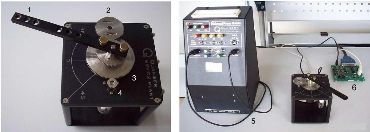
Figure 2. Quanser servo positioning arm platform: 1) arm; 2) potentiometer; 3) main shaft + encoder; 4) electric motor + gear box; 5) power module; 6) acquisition board.
