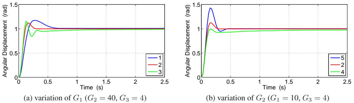
Figure 9. Unitary step response of the servo positioning system with chosen gains from the volume in the space of gains (experimental results).
