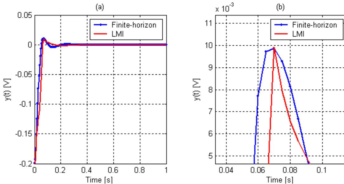
Figure 6. (a) Comparison of the presented solutions:  $K_{real} = 0.90K_{nominal}$  with robust treatment. (b) Constraint detail.
