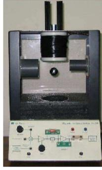
Figure 1. Feedback™ magnetic levitation system.
