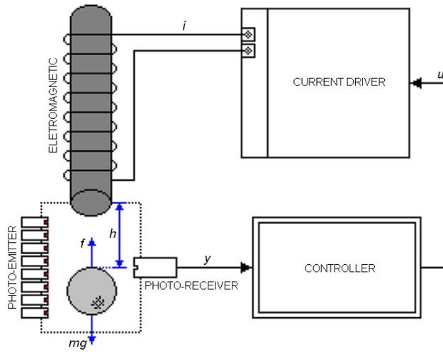
Figure 2. Control loop schematic.  $f$  denotes the attraction force related to  $i$  and  $h$ .
