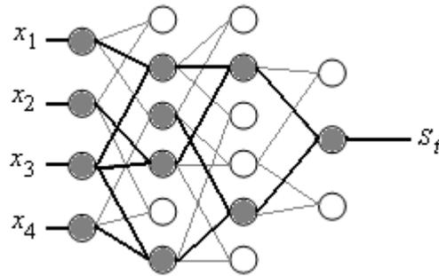
Figure 1. Example of neural network structure obtained by GMDH algorithm.
