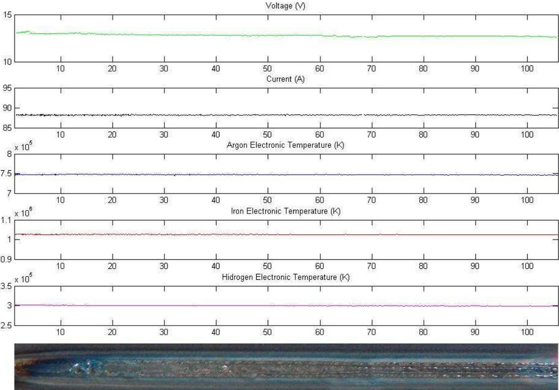
Figure 5 – Electronic Temperature in a plate without defects.
