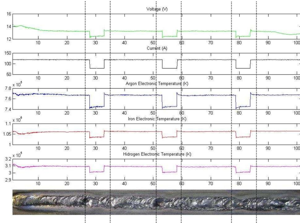
Figure 8 - Experiment with current defect of 1 second
