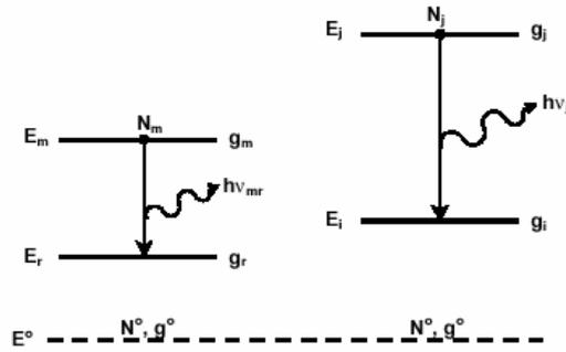
Figure1 - Spectra lines at the same ionization stage
