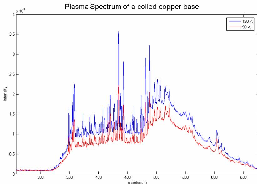
Figure 3 – GTAW spectrum on a cooled copper plate
