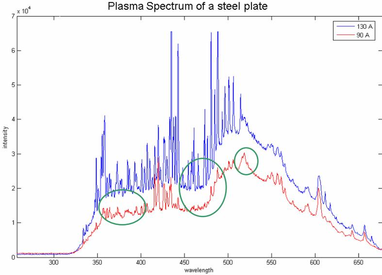
Figure 4 – GTAW spectrum on a steel plate.
