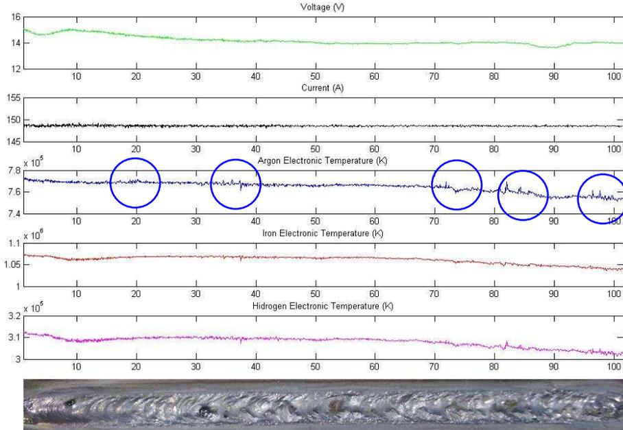
Figure 6 - Defect on shielding gas flow rate
