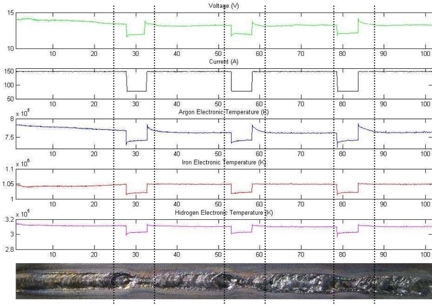
Figure 7 - Experiment with current defect of 2 seconds
