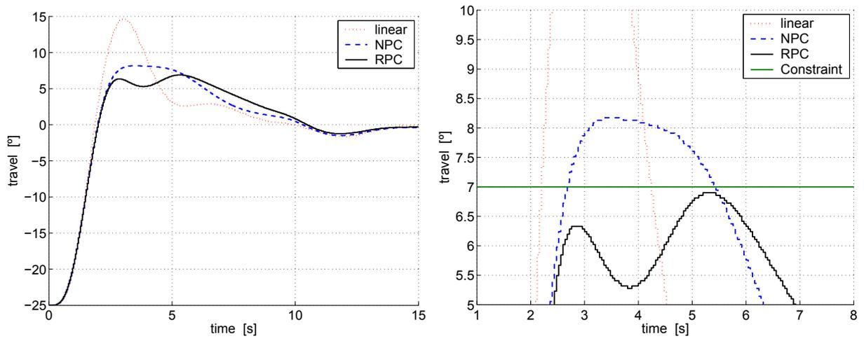
Figure 5. Travel angle ( $x_5$ ) during maneuver and detail of travel constraint violation (at 7 degrees) by the nominal linear and NPC control laws.
