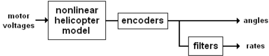
Figure 2. Block diagram of the helicopter simulation model.
