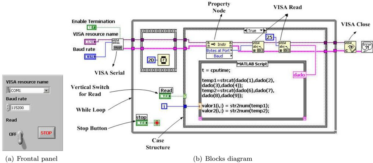
Figure 6. Windows developed in the LabVIEW software.
