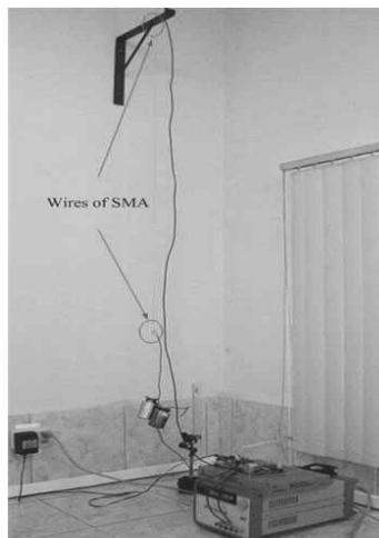
Figure 3. Experimental set-up for thermomechanical training of the SMA wire.
