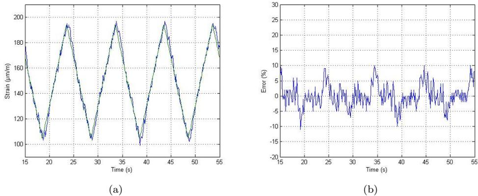
Figure 9. Experimental results using controller PI for triangular reference.
