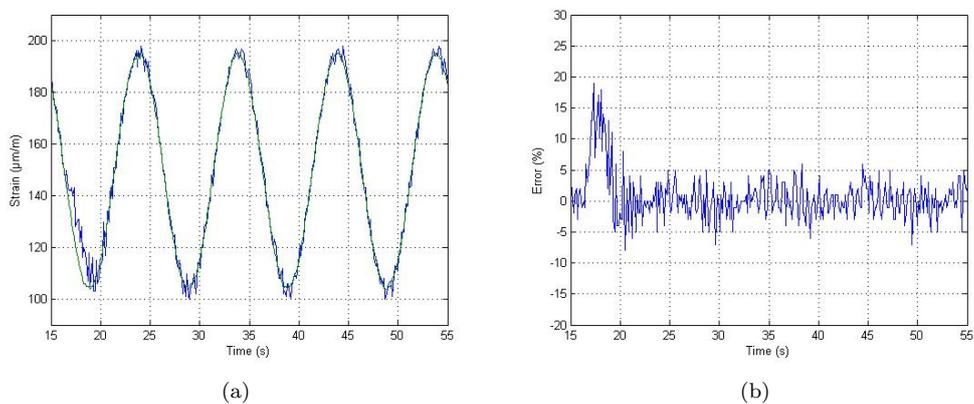
Figure 10. Experimental results using controller PI for sinusoidal reference.
