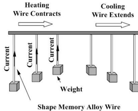
Figure 2. SMA wire working as an actuator.
