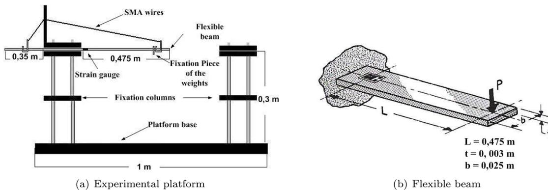
Figure 4. Diagram of the experimental platform.
