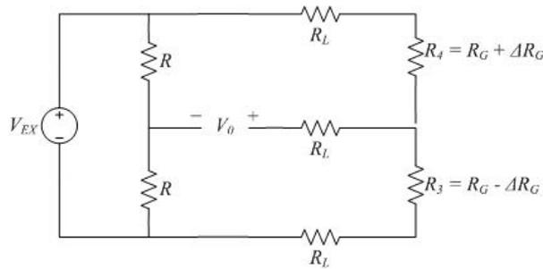
Figure 1. Electrical design of the Wheatstone bridge.
