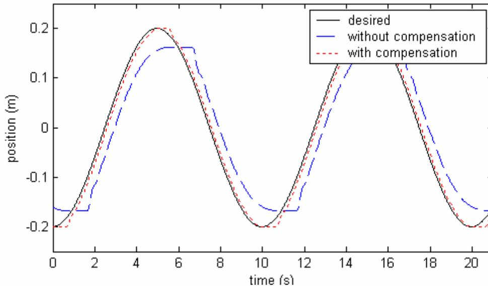
Figure 4. Experimental results to sinusoidal trajectory tracking
