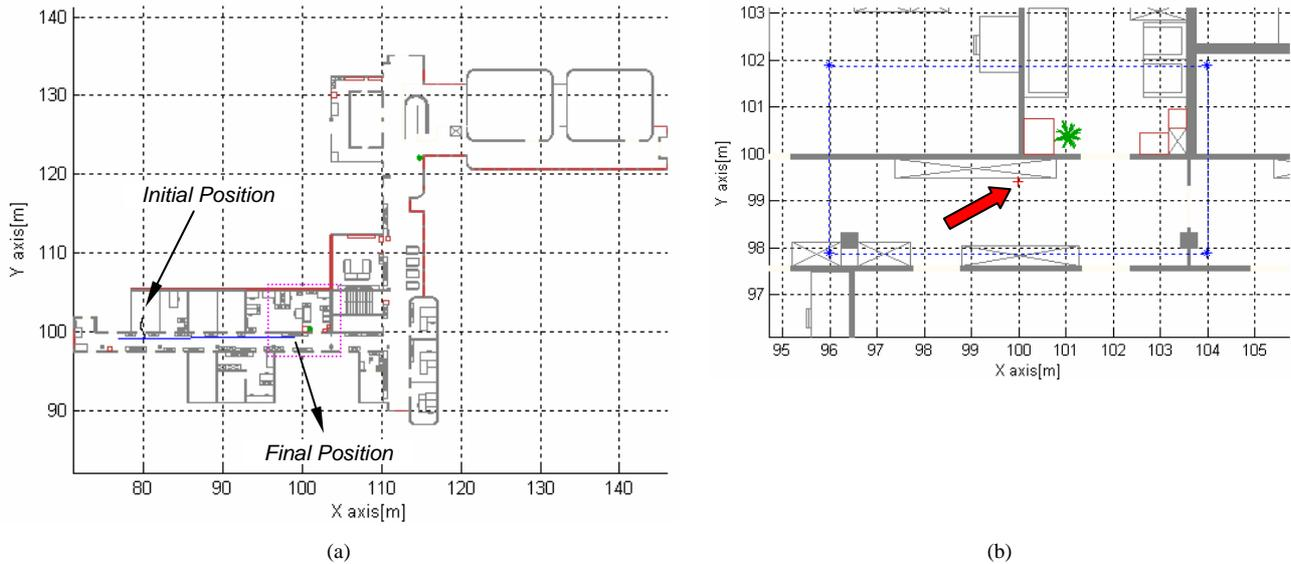
Figure 7. Trajectory estimation obtained from fusion of system state predictions by laser scan data and omni-directional camera images (a) and final robot position found.
