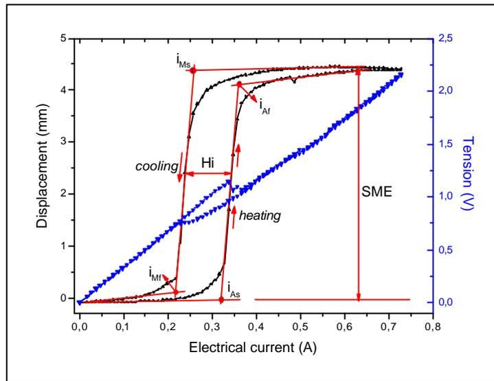
Figure 4 – Main electromechanical shape memory parameters. TN1 specimen under 200MPa.
