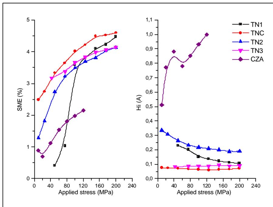
Figure 6 – Shape memory effect and current hysteresis versus applied stress.
