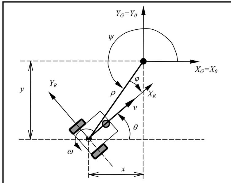
Figure (2): Configuration of the kinematic control.
