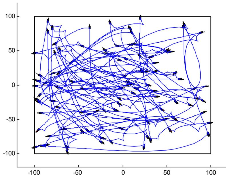
Figure (4): The mobile robot trajectory to achieve 100 planned points using continuous control law (control gains  $k_1=1.5$  and  $k_2=5.5$ ).
