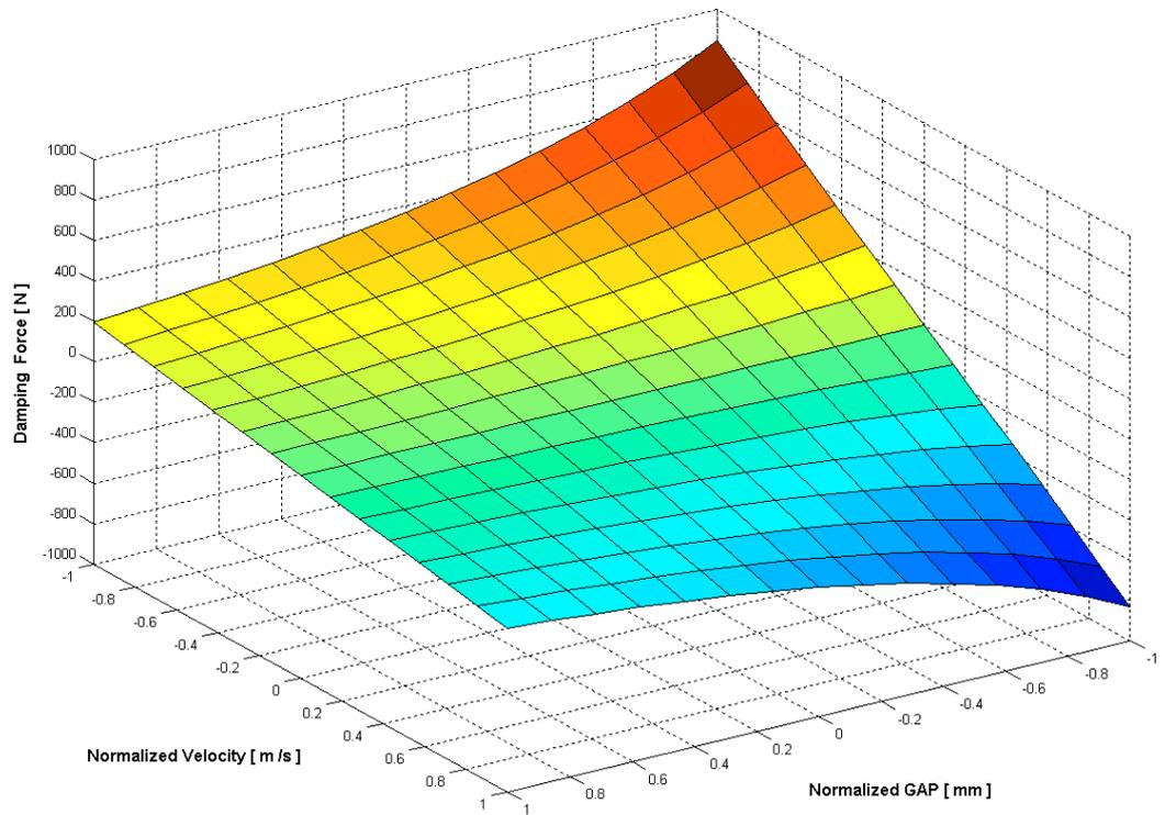
Figure 13. Neural-fuzzy model for the damping Force.
