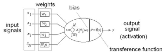
Figure 6: A processing element.
