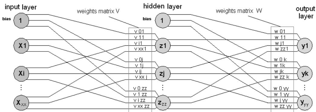
Figure 5: A backpropagation neural network with 1 hidden layer.
