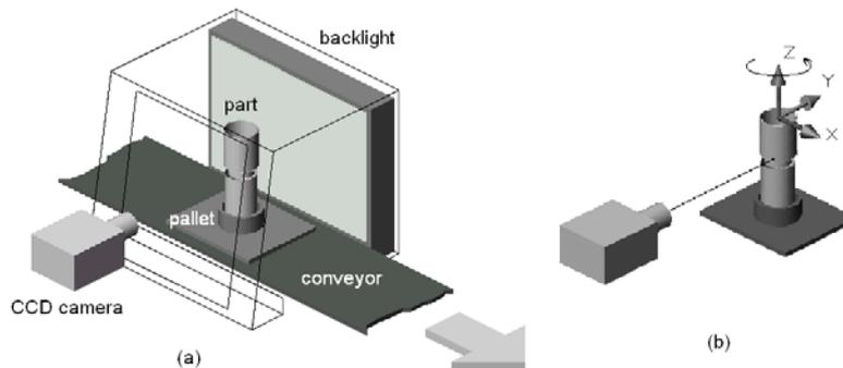
Figure 2: (a) The inspection cabin for image acquisition. (b) A coordinate system fixed on the part.
