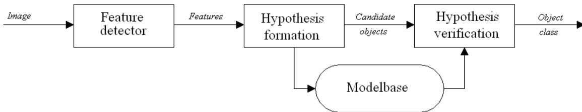
Figure 1: The ORVS block diagram (Jain, 1995)
