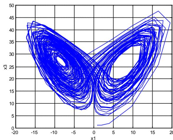
Figure 2: The  $x_1x_3$  phase plan of Lorenz system.
