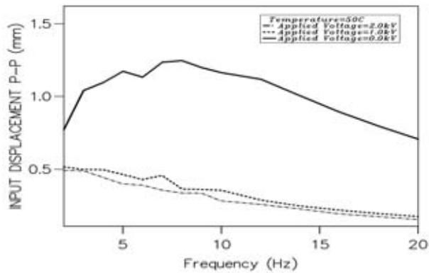
Figure 4: Input Displacement versus Frequency
