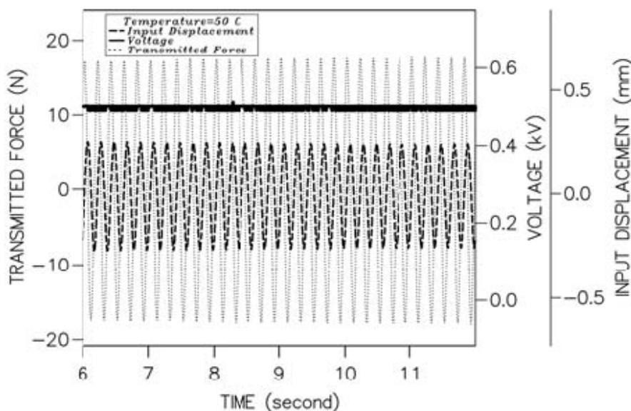
Figure 9: Responses to Step Change in Voltage
