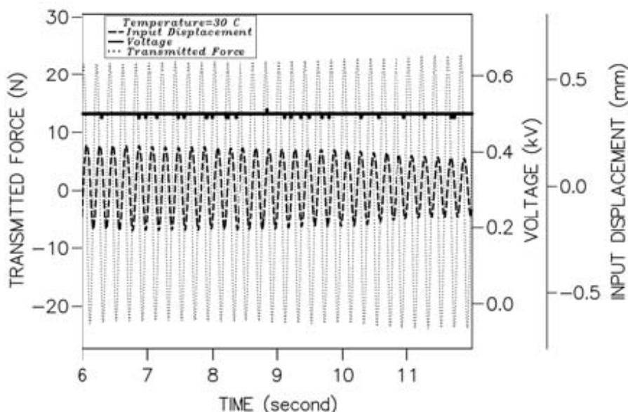
Figure 7: Responses to Step Change in Voltage
