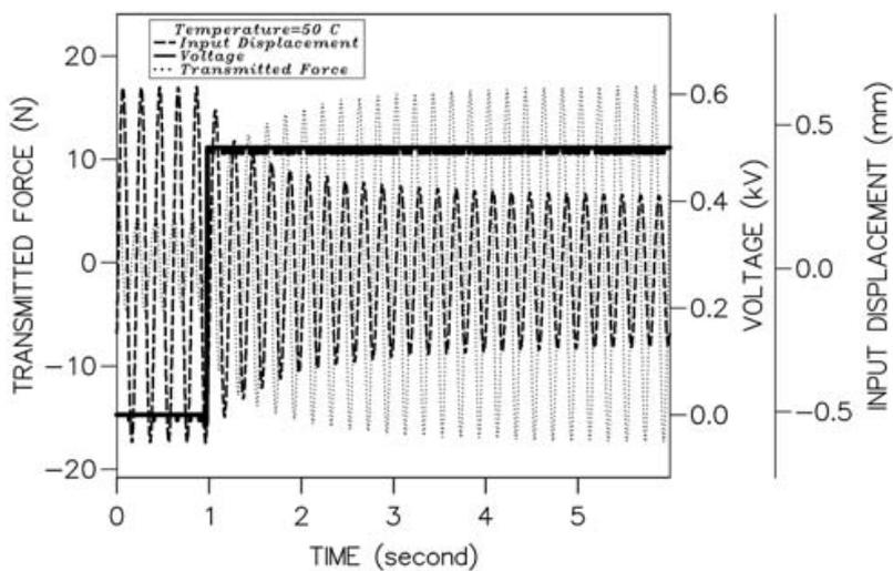
Figure 8: Responses to Step Change in Voltage
