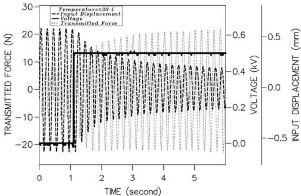
Figure 6: Responses to Step Change in Voltage
