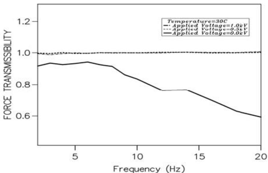
Figure 3: Force Transmissibility v Frequency
