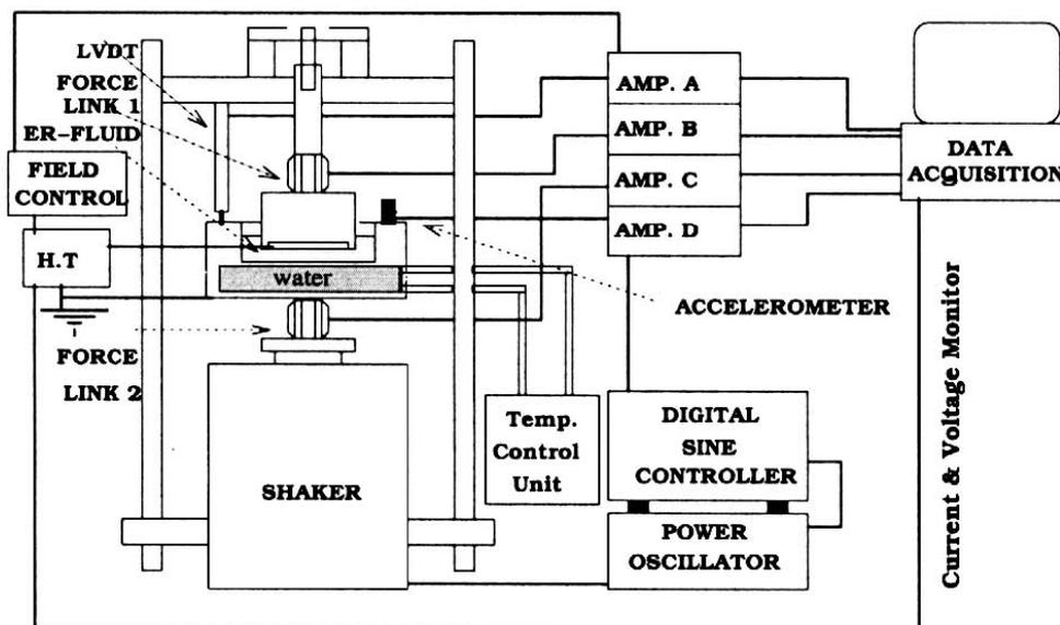
Figure 1: Experimental Arrangement.
