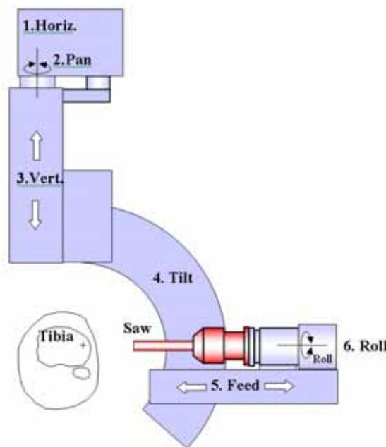
Figure.3: Kinematic configuration of the active manipulator
