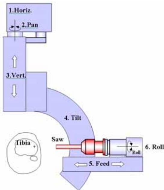
Figure.3: Kinematic configuration of the active manipulator
