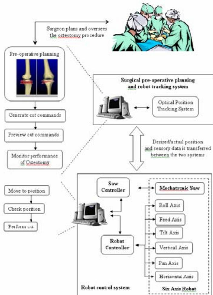
Figure 2: Mechatronic Assisted Osteotomy.
