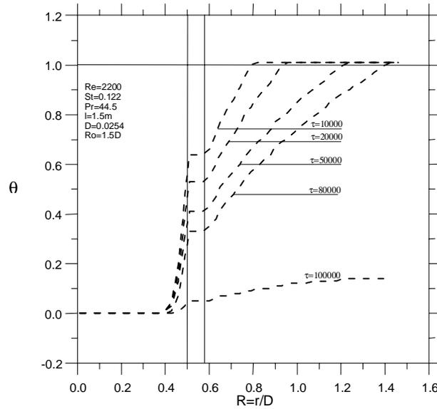
Figure 3- Radial temperature distribution at the middle of the pipe for different time periods.
