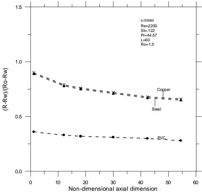
Figure 9- Solidification front position as function of tube wall materials.
