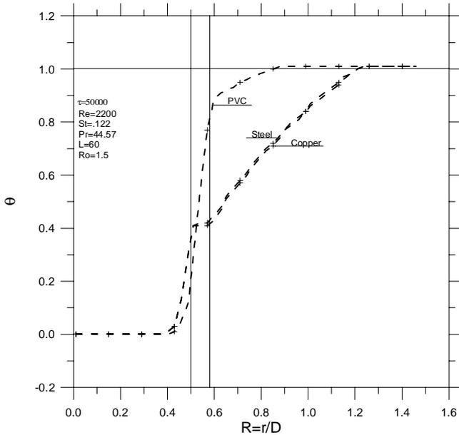
Figure 8- Radial temperature distribution for different tube wall materials.
