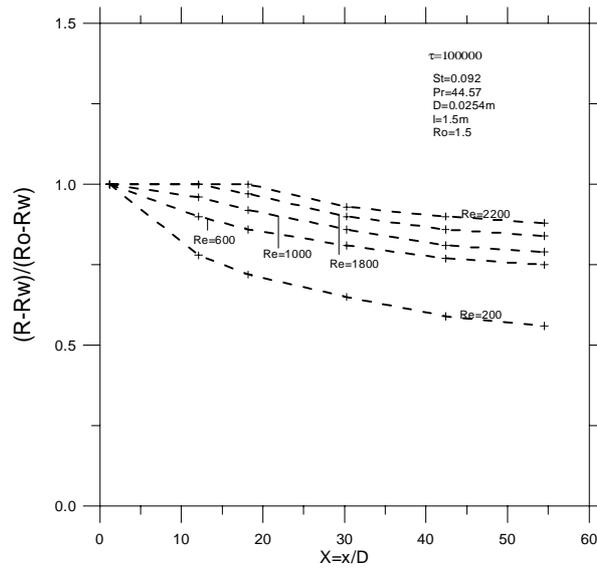
Figure 5- Position of the solidification front for different Reynolds numbers.
