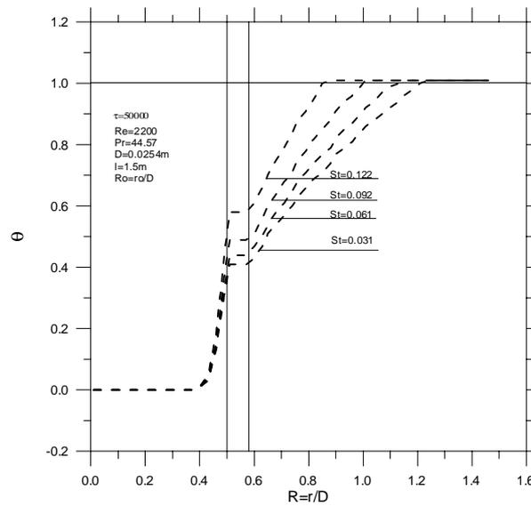
Figure 6 - Radial temperature distribution for different Stefan numbers
