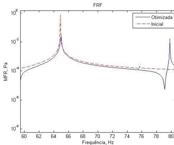
Figure 4: Sound pressure initial and optimized for 60-80 Hz interval using genetic algorithm
