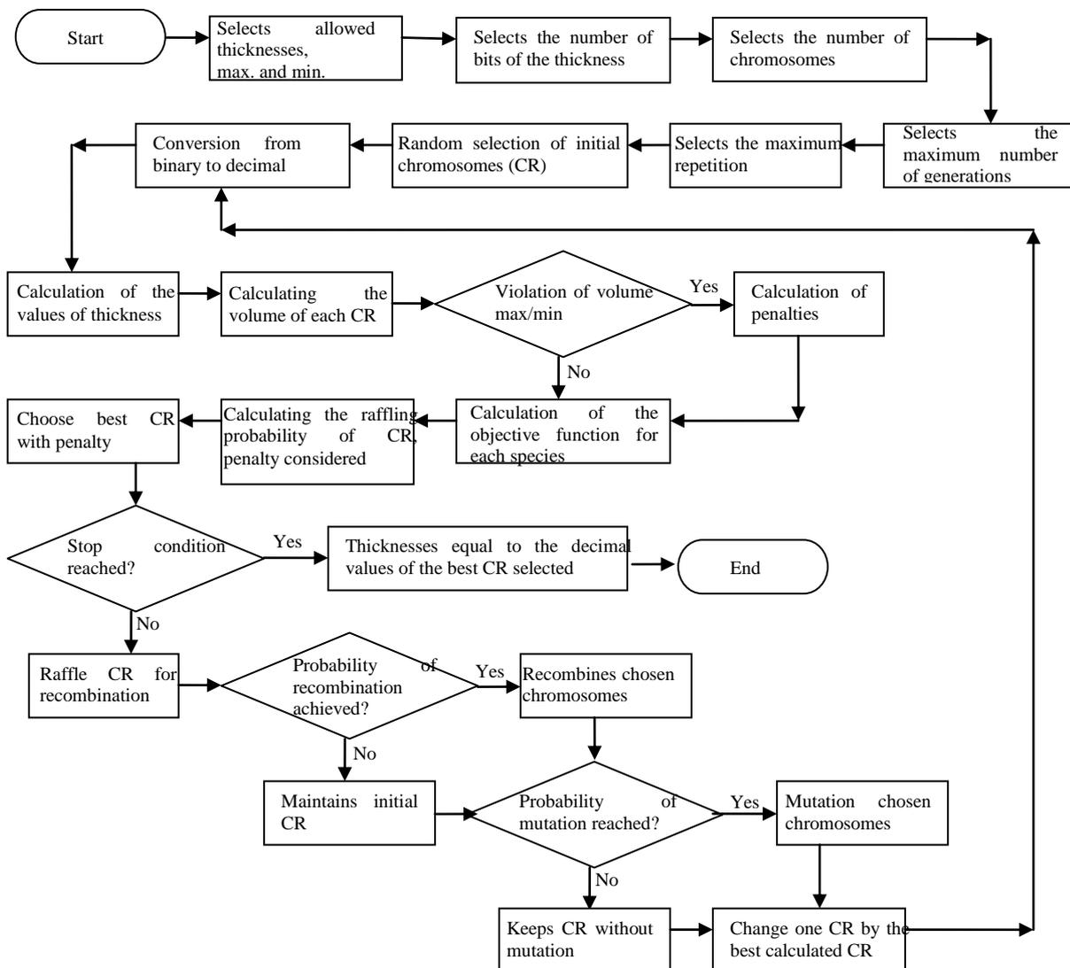
Figure 1: Flowchart of the optimization process with Genetic Algorithms
