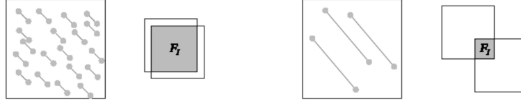
Figure 2.9: The number of particle-image pairs that can be contained in an interrogation region is reduced for increasing displacement (Westerweel, 1997).
