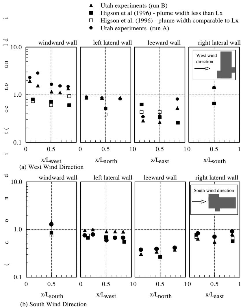
Figure 6 – Concentration fluctuation intensity in neutral conditions for a source located upwind of the centre of (a) the long face of the building and (b) the short face of the building. The two different symbols represent two periods of 5 minutes in similar meteorological conditions.
