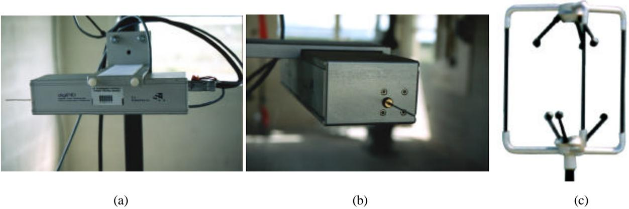
Figure 2 – (a) Lateral and (b) frontal views of a PID detector, manufactured by Aurora Scientific Inc. (c) The ultra-sonic anemometer sensor system.
