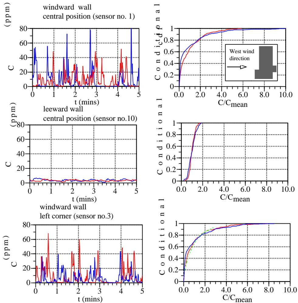
Figure 7 – Time series and conditional cdf's in neutral condition for source located upwind of the centre of the long face of the building. The two different experiments (run A and run B) represent two periods of 5 minutes in similar meteorological conditions.
