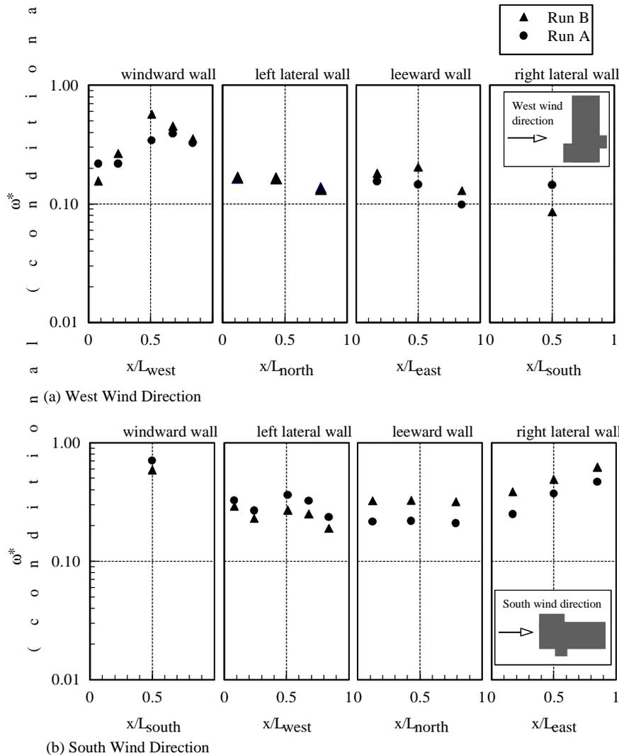
Figure 5 – Mean concentration in neutral conditions for source located upwind of the centre of (a) the long face of the building and (b) short face of the building. The two different symbols represent two periods of 5 minutes in similar meteorological conditions.
