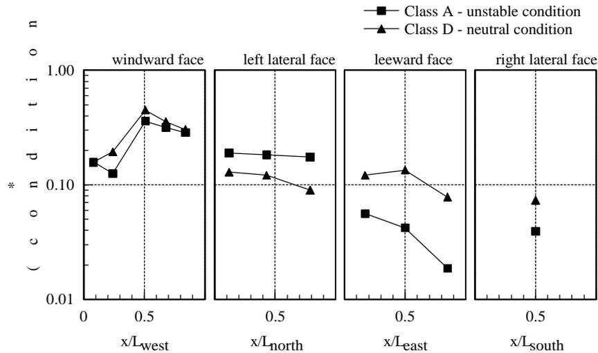
Figure 9 – Conditional mean concentration on the building surface for neutral and unstable atmospheric stability conditions.
