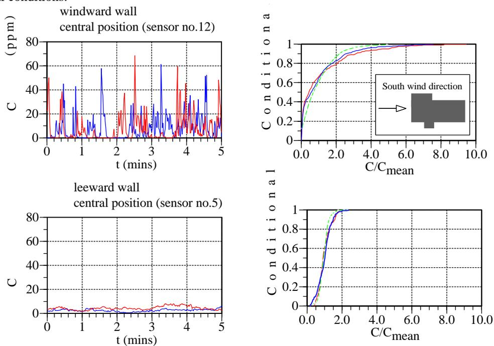
Figure 8 - Time series and conditional cdf's in neutral condition for source located upwind of the centre of the short face of the building. The two different experiments (run A and run B) represent two periods of 5 minutes in similar meteorological conditions.
