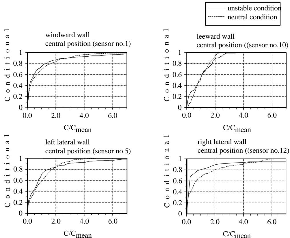
Figure 11 – Conditional cdf's on the building surface for neutral and unstable atmospheric conditions.
