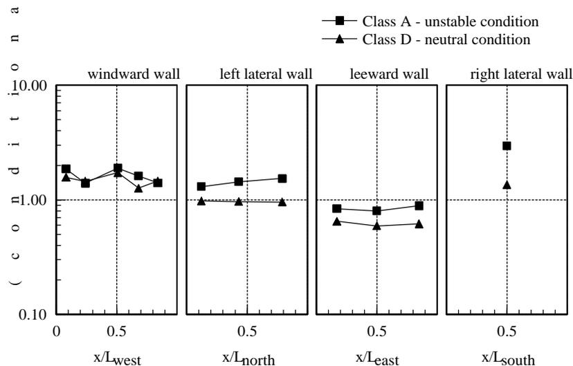
Figure 10 – Conditional concentration fluctuation intensity on the building surface for neutral and unstable atmospheric conditions.
