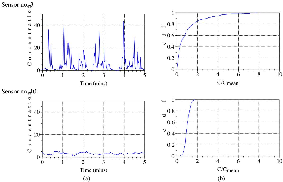
Figure 3 – Examples of (a) time series and (b) cdf's for two different positions around the obstacle.
