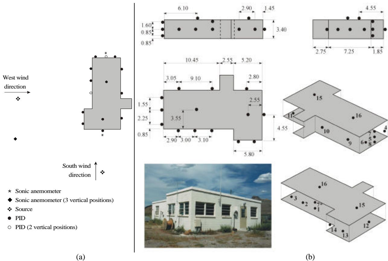
Figure 1 – (a) Schematic representation of the site, (b) the building used in the experiments at Dugway Proving Ground (view looking from SSW) and a schematic representation of the sensor locations on the building surfaces.
