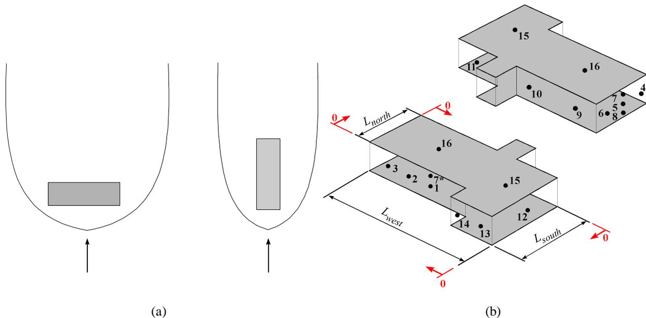
Figure 4 – (a) Schematic representation of the regions around the obstacle in which the flow is influenced by the building presence in the case of wider and longer obstacle. (b) Schematic representation of the lengths  $L_{west}$ ,  $L_{north}$ ,  $L_{south}$ .
