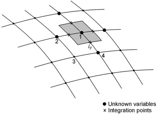
Figure 6 – Cell-vertex construction without using the element
