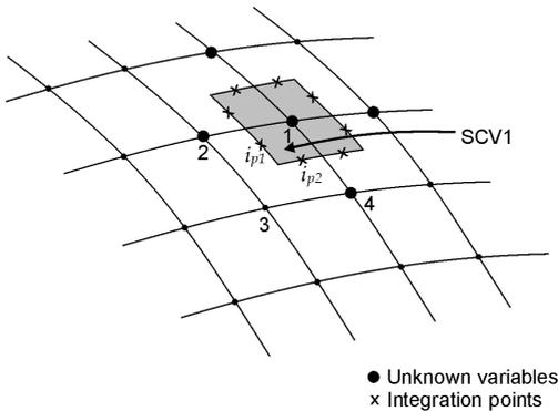
Figure 7- Cell-vertex construction using the element
