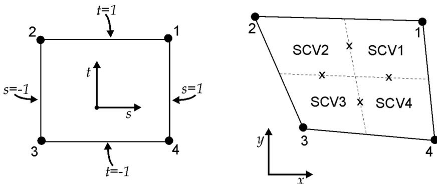
Figure 10 – Transformed  $(s,t)$  and physical  $(x,y)$  domains.
