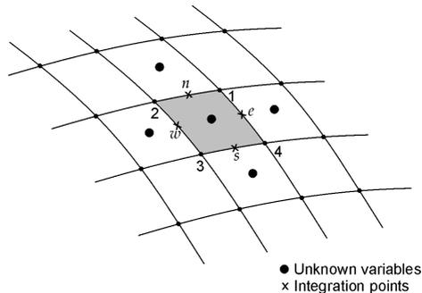
Figure 5 – Control volume coincident with the element in the classical finite volume method
