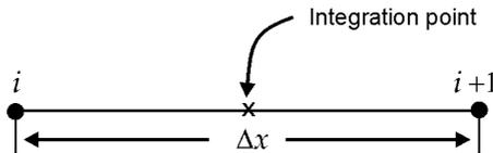
Figure 11 – 1D example for the construction of the interpolation function (Raw, 1985)
