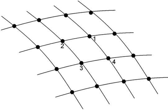
Figure 3 – Structured curvilinear grid
