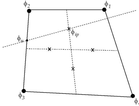
Figure 12 –Determination of  $\phi$  at the integration point
