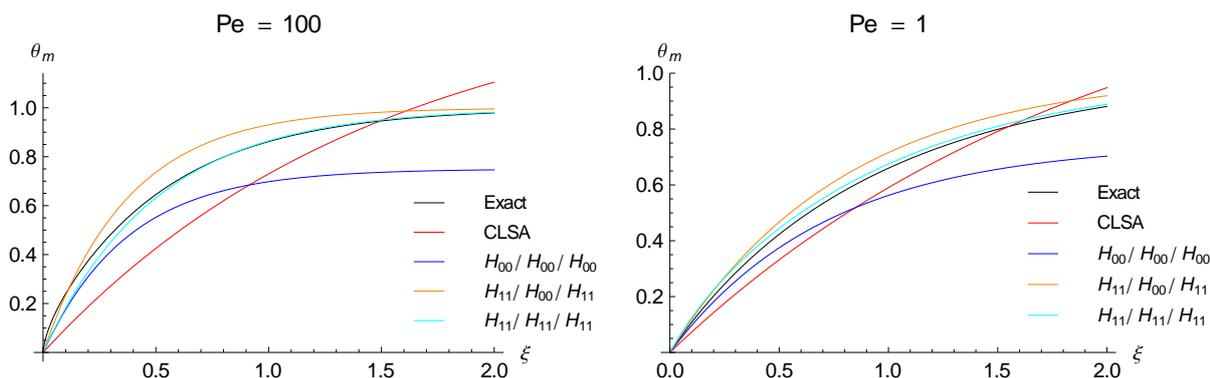
Figure 2. Comparison between different lumped approximation schemes and exact solution for different Péclet numbers for a laminar flow.
