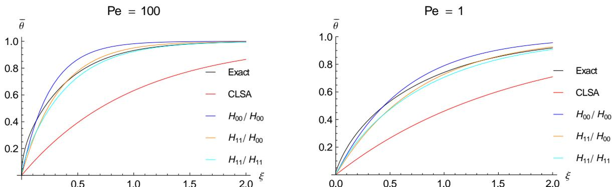
Figure 1. Comparison between different lumped approximation schemes and exact solution for different Péclet numbers.
