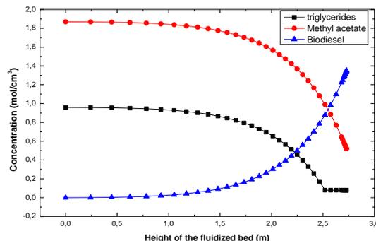
Figure 1. The concentration of triglycerides, methyl acetate and biodiesel.
