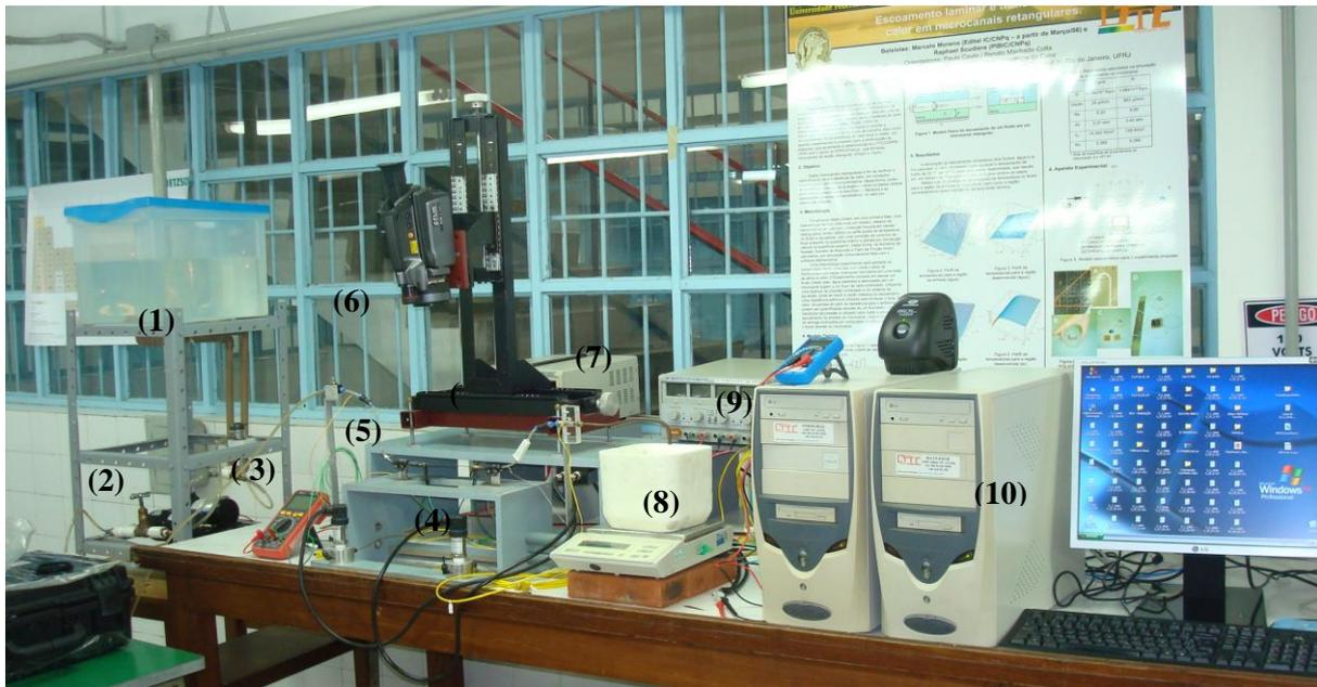
Figure 1. Overall view of the experimental setup for forced convection analysis in micro-needles.
