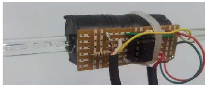
Figure 2: Optical Sensor.
