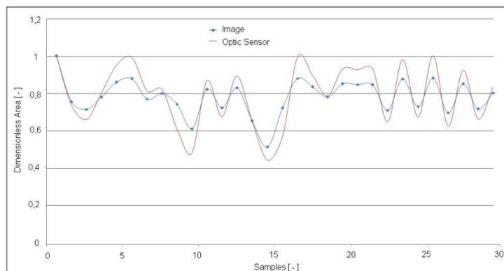
Figure 9: Comparison area's image with area's optical sensor.
