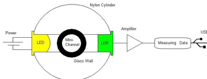
Figure 1: Block diagram of the optical sensor.
