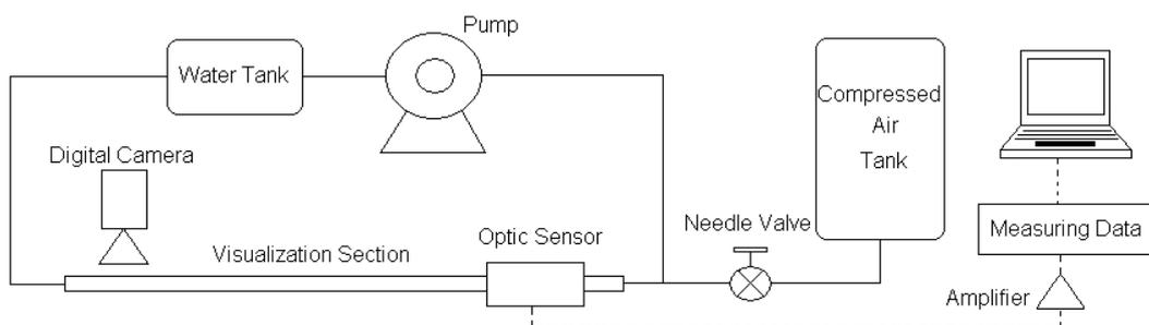
Figure 3: Schematic diagram of experimental apparatus.
