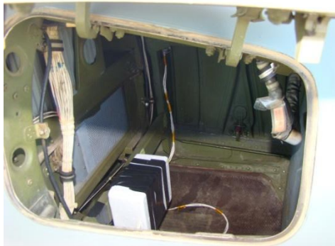
Figure 2.c. Insulated data logger in the front compartment.
