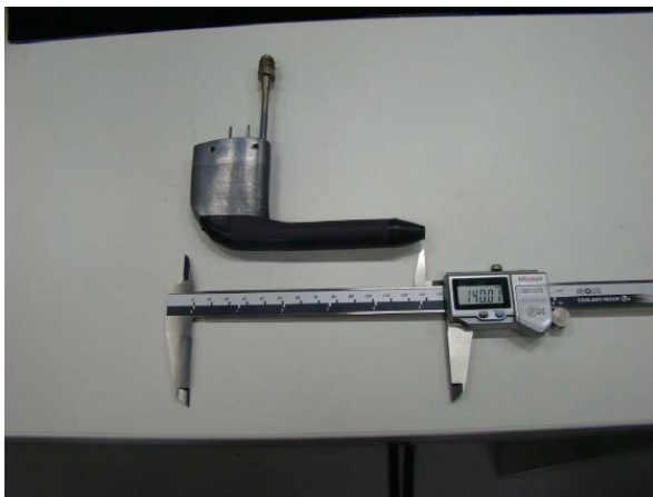
Figure 1.a. A4 Skyhawk Pitot tube, manufactured by AeroInstruments Co., USA.
