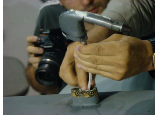
Figure 2.b. Installation of the Pitot tube on the aircraft.
