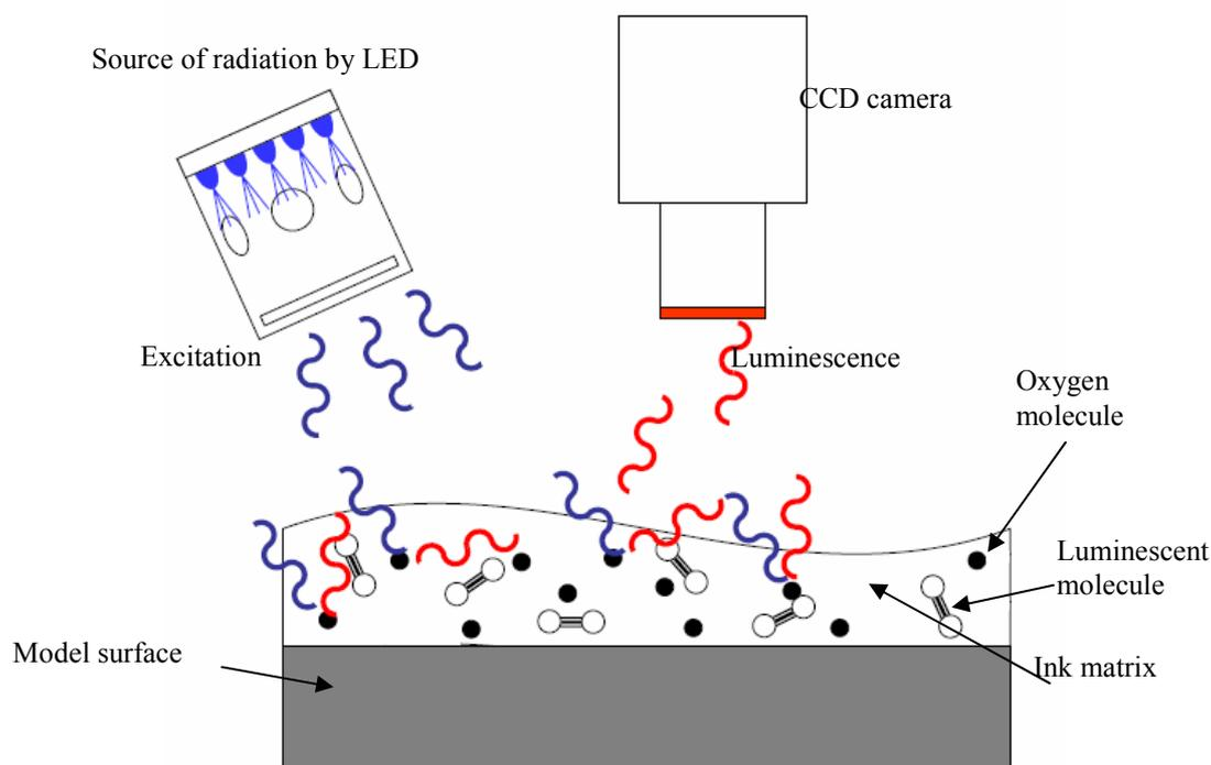
Figure 4. Physical principle of the PSP technique.
