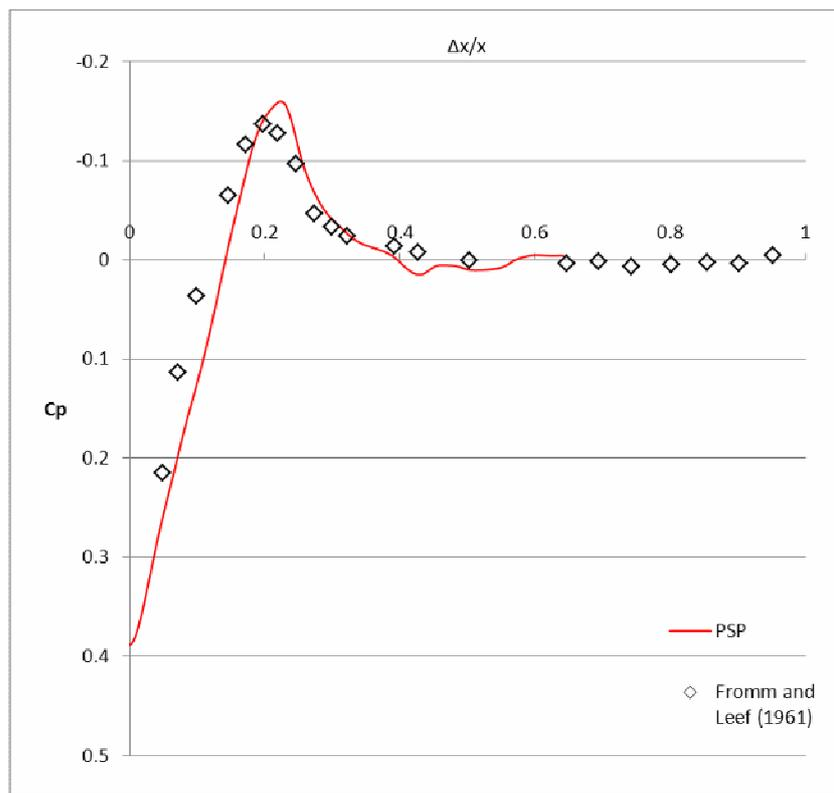
Figure 5. Dimensionless pressure coefficient distribution along surface of AGARD-C test model obtained with PSP technique, freestream Mach number 0.6, and blockage ratio of 0.8% compared to model from calibrated tunnel, measured with pressure taps and 0.4% of blockage.
