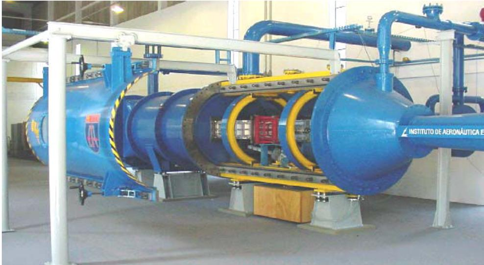
Figure 1. Pilot Transonic Wind Tunnel installation – plenum chamber door open.
