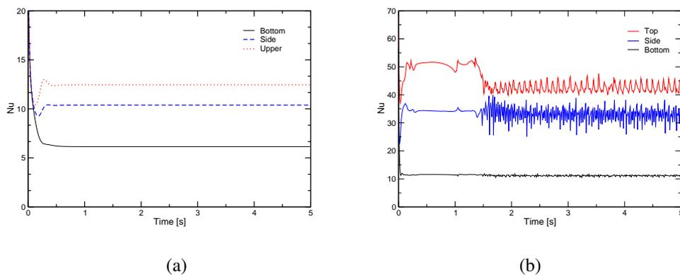
Figure 2. Boundary averaged Nusselt provided by LS model for  $Pr = 0.6$  at (a)  $Ra = 10^6$  and (b)  $Ra = 10^9$
