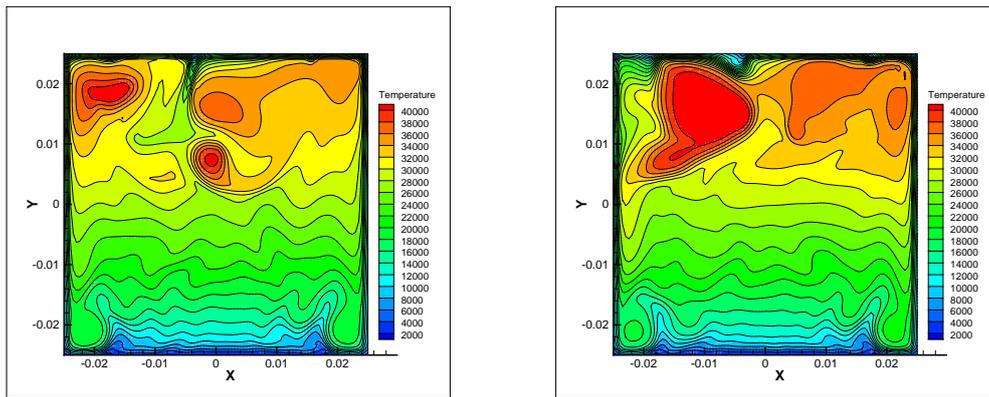
Figure 3. Temperature field computed with SST for  $Pr = 0.6$  and  $Ra = 10^{11}$  at (a) 1500s and (b) 6000s
