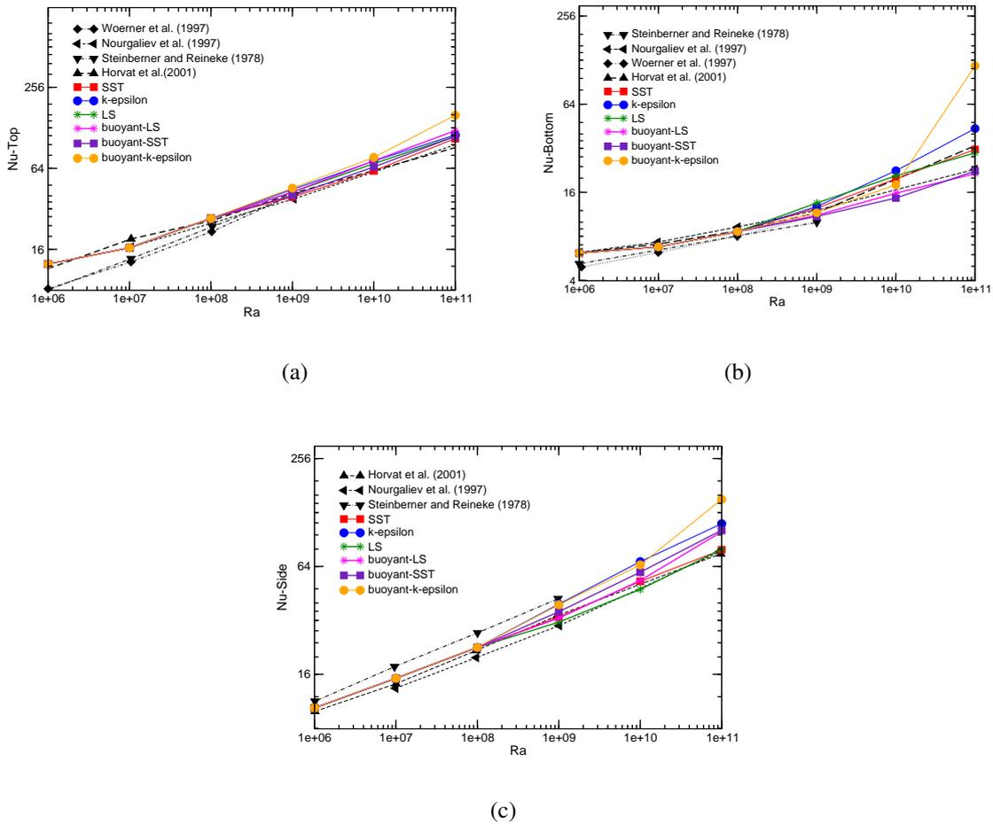
Figure 5. Average Nusselt numbers as a function of Ra numbers for  $Pr = 0.6$  at : (a) the top wall, (b) the bottom wall and (c) the side wall.
