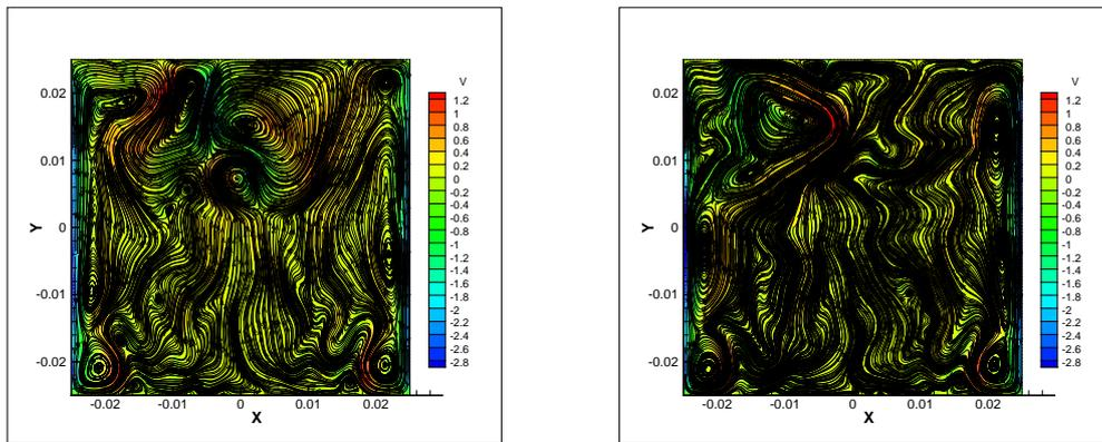
Figure 4. Vertical velocity field computed with SST for  $Pr = 0.6$  and  $Ra = 10^{11}$  at (a) 1500s and (b) 6000s
