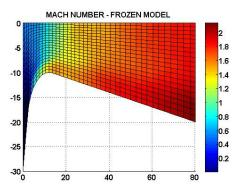
Figure 6. Temperature and Mach number distribution along the nozzle for the frozen model.
