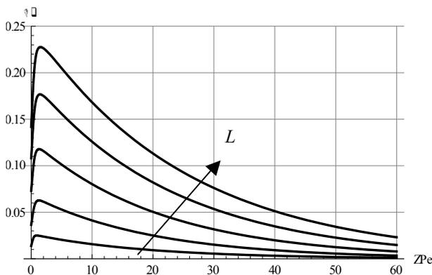
Figure 3. Difference between the internal and external wall temperatures along the channel length for five different wall thicknesses ( $L = 900, 650, 400, 200, 75 \mu\text{m}$ ) – steady state.
