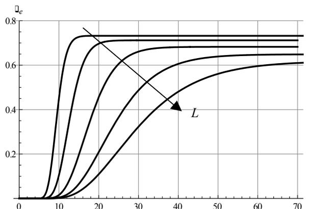
Figure 5. Time evolution of the external wall temperature at  $ZPe = 5$  for five wall thicknesses ( $L = 900, 650, 400, 200, 75 \mu\text{m}$ ).
