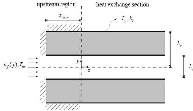
Figure 1. Schematic representation of the conjugate heat transfer problem in a micro-channel with upstream region.
