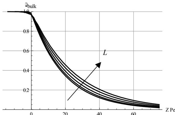
Figure 2. Fluid bulk temperature along the channel length for five different channel wall thicknesses ( $L = 900, 650, 400, 200, 75 \mu\text{m}$ ) – steady state.
