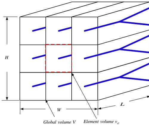
Figure 1a. Three-dimensional Y-shaped channels across a solid body with internal heat generation
