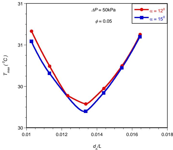
Figure 2. Effect of optimised hydraulic diameter  $d_h$ , on the peak temperature
