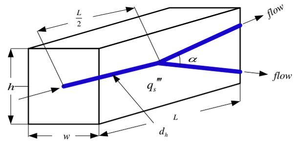
Figure 1b. The three dimensional computational domain of elemental volume with Y-shaped cooling channel
