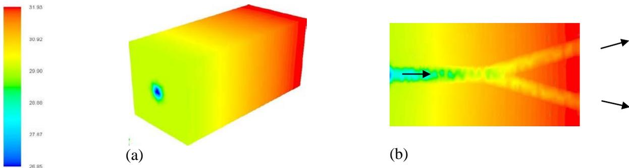
Figure 4. Temperature distributions (a) on the unit structure and (b) on the cooling fluid and inner wall.
