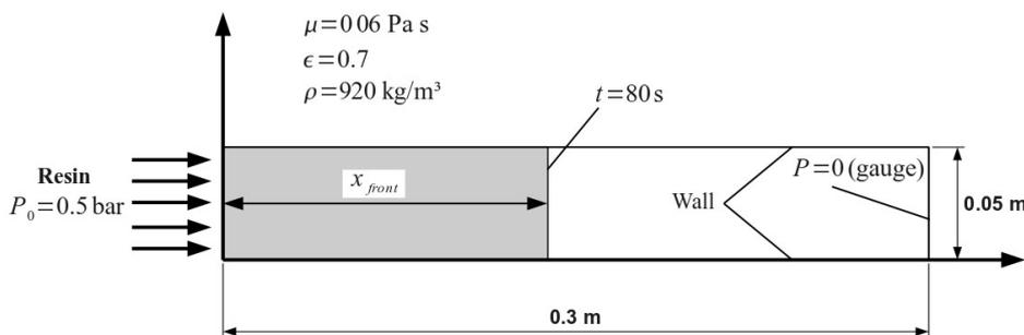
Fig. 2 - Computational domain for the rectilinear solution sumiu um “.” de 0.06
