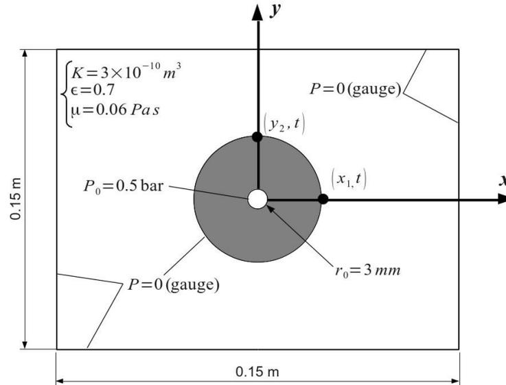
Fig. 3 - Computational domain for the radial 2D solution
