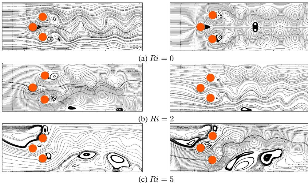
Figure 3. Streamlines for (a)  $Ri = 0$ , (b)  $Ri = 2$  and (c)  $Ri = 5$ . Left column  $S_h = 2.5d$  and  $S_v = 1.25d$ . Right column  $S_h = 3d$  and  $S_v = 1.5d$
