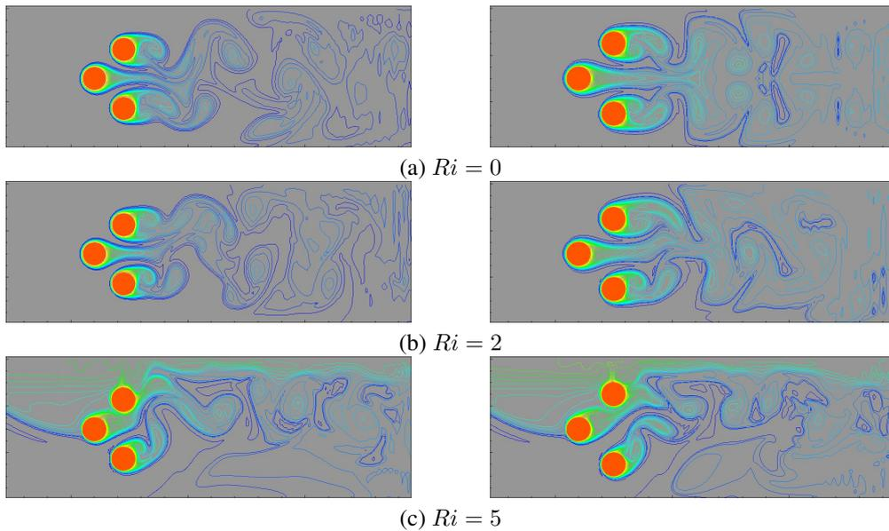
Figure 2. Instantaneous Isotherms for (a)  $Ri = 0$ , (b)  $Ri = 2$  and (c)  $Ri = 5$ . Left column  $S_h = 2.5d$  and  $S_v = 1.25d$ . Right column  $S_h = 3d$  and  $S_v = 1.5d$ .
