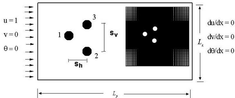
Figure 1. Computational domain and boundary conditions for case 1.
