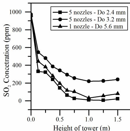
Figure 6. Influence of the height of the tower on SO<sub>2</sub> concentration.
