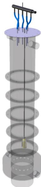
Fig 3: Probe for sample collection inside of the tower.
