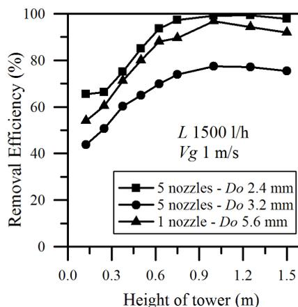
Fig. 7: Influence of the height of the tower on the removal efficiency of SO<sub>2</sub>.
