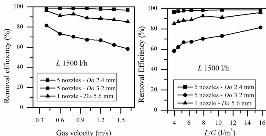
Figure 4. Influence of the gas velocity and  $L/G$  on the removal efficiency of  $SO_2$ .
