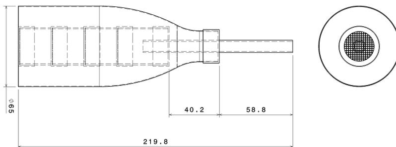
Figure 2. Probe to collect gas sample.
