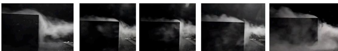
Figure 13. Side view of the incident flow around rectangular prismatic building ( $L/H = 2.0$ ) at  $Re = 1.5 \times 10^4$ .
