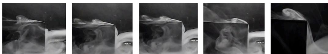
Figure 10. Side view of the incident flow rectangular prismatic building ( $L/H = 2.0$ ) at  $Re = 1.8 \times 10^3$ .
