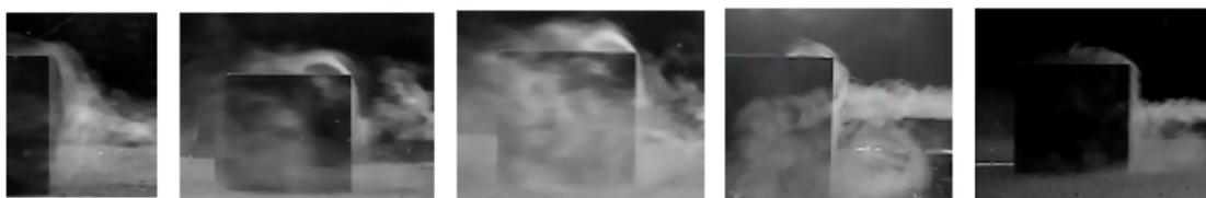
Figure 4. Side view of the incident flow around cubic building ( $L/H = 1.0$ ) at  $Re = 7.1 \times 10^3$ .
