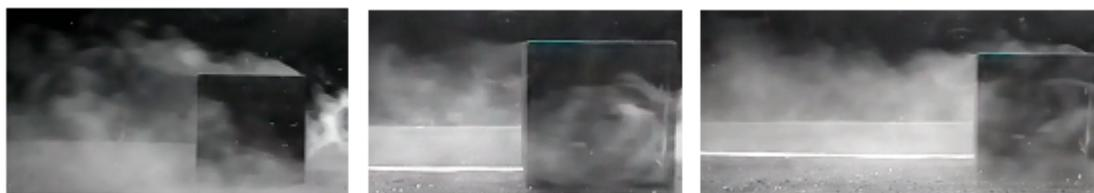
Figure 8. Side view of the flow in near wake around cubic building ( $L/H = 1.0$ ) at  $Re = 7.1 \times 10^3$ .
