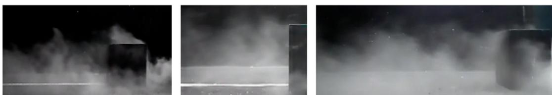
Figure 9. Side view of the flow in near wake around cubic building ( $L/H = 1.0$ ) at  $Re = 1.5 \times 10^4$ .
