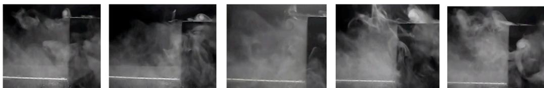
Figure 7. Side view of the flow in near wake around cubic building ( $L/H = 1.0$ ) at  $Re = 3.2 \times 10^3$ .
