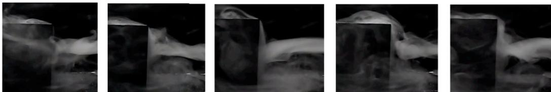
Figure 3. Side view of the incident flow around cubic building ( $L/H = 1.0$ ) at  $Re = 3.2 \times 10^3$ .
