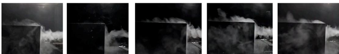
Figure 12. Side view of the incident flow around rectangular prismatic building ( $L/H = 2.0$ ) at  $Re = 7.1 \times 10^3$ .
