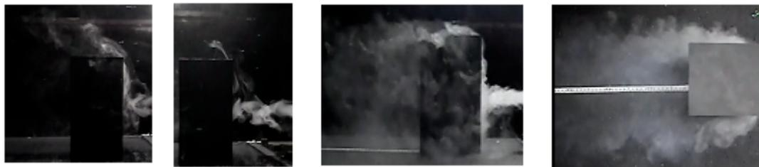
Figure 17. View of the flow in the vicinity of the rectangular prismatic building ( $L/H = 0.5$ ) at  $Re = 8.8 \times 10^3$ .
