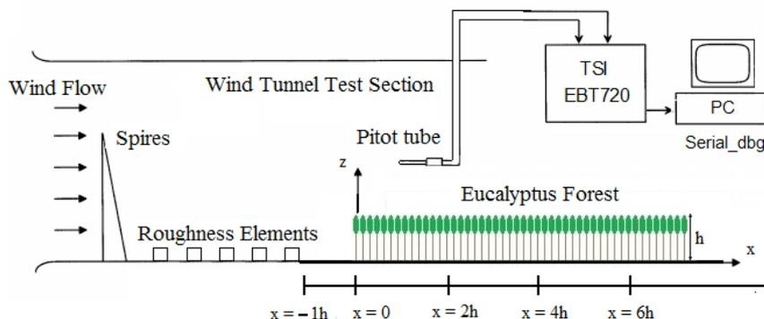
Figure 1. Sketch of the wind tunnel test section, measurement system and forest localization.
