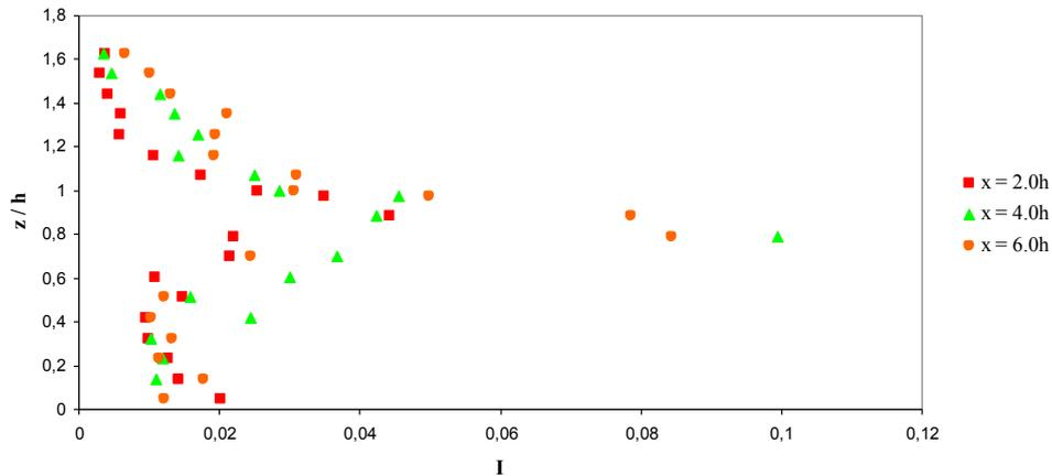
Figure 6. Vertical profiles of turbulence intensity within and above the forest region at  $Re = 3.4 \times 10^4$ .
