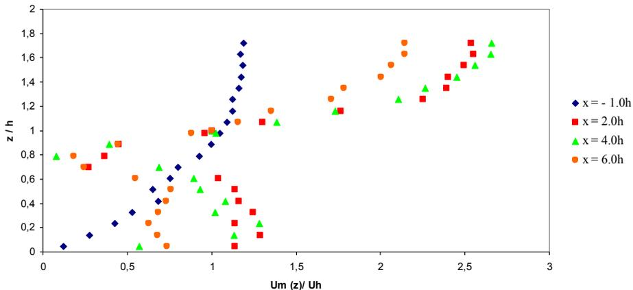
Figure 3. Normalized vertical profiles of mean wind velocity normalized at  $Re = 2.8 \times 10^4$ .
