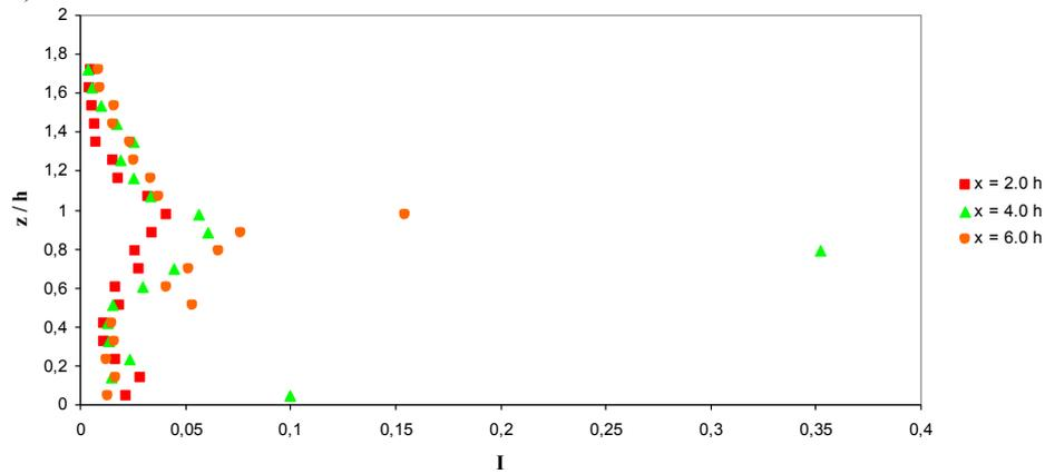
Figure 5. Vertical profiles of turbulence intensity within and above the forest region at  $Re = 2.8 \times 10^4$ .
