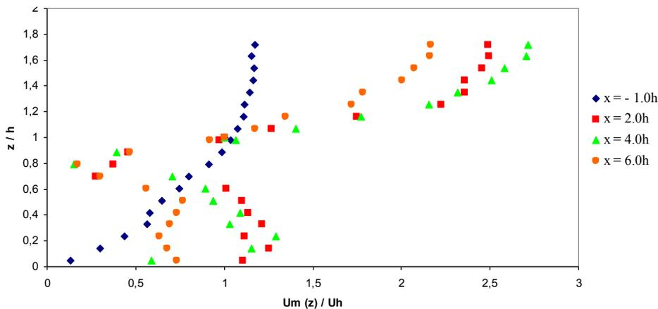
Figure 4. Normalized vertical profiles of mean wind velocity normalized at  $Re = 3.4 \times 10^4$ .
