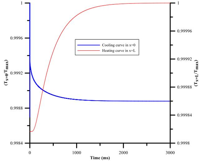
Figure 2. Transient evolution of the temperature in the anterior and posterior surfaces of the sample
