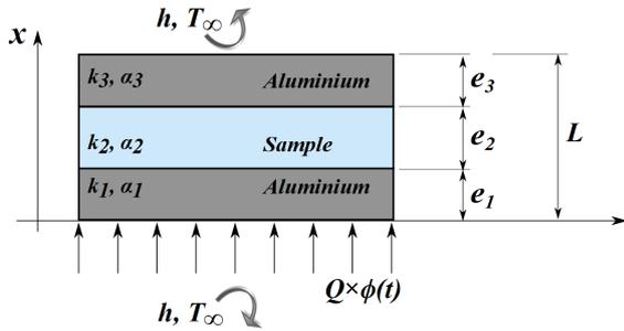
Figure 1. Representation of the physical model
