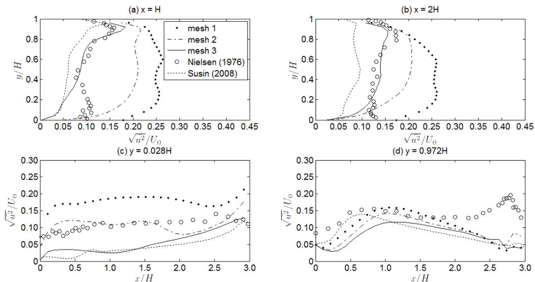
Figure 4. Dimensionless turbulent intensity in the symmetry plan.
