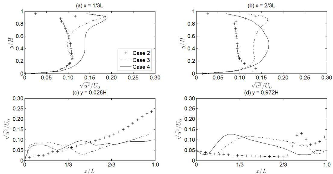
Figure 8. Dimensionless mean turbulent intensity in the symmetry plan, for cases 2, 3 and 4.
