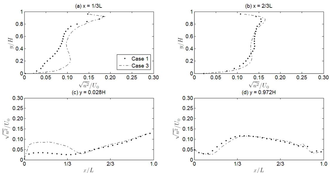
Figure 6. Dimensionless mean turbulent intensity in the symmetry plan, for cases 1 and 3.
