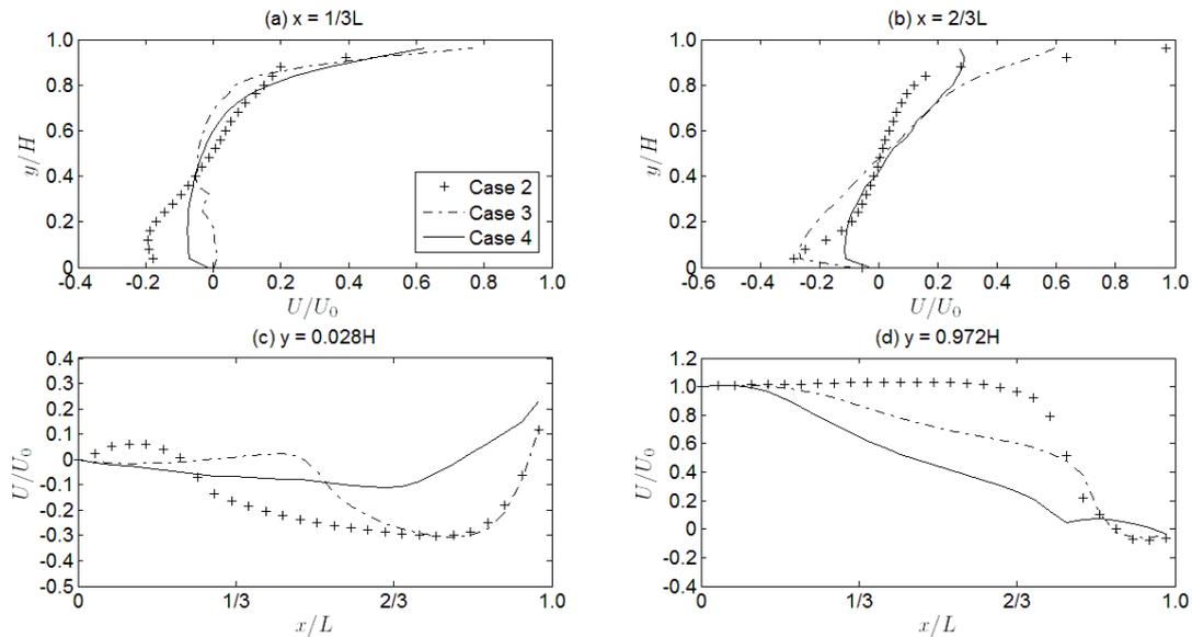
Figure 7. Dimensionless mean velocity in the symmetry plan, for cases 2, 3 and 4.
