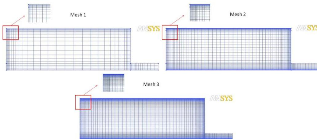
Figure 2. Lateral section of the three meshes used in case 1.
