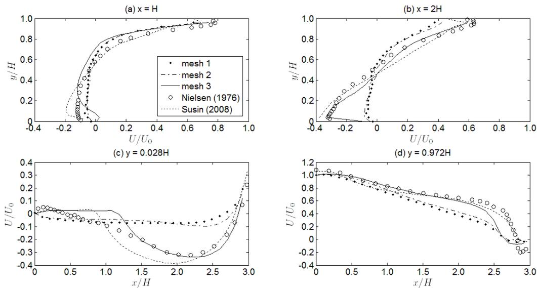
Figure 3. Dimensionless mean velocity in the symmetry plan.
