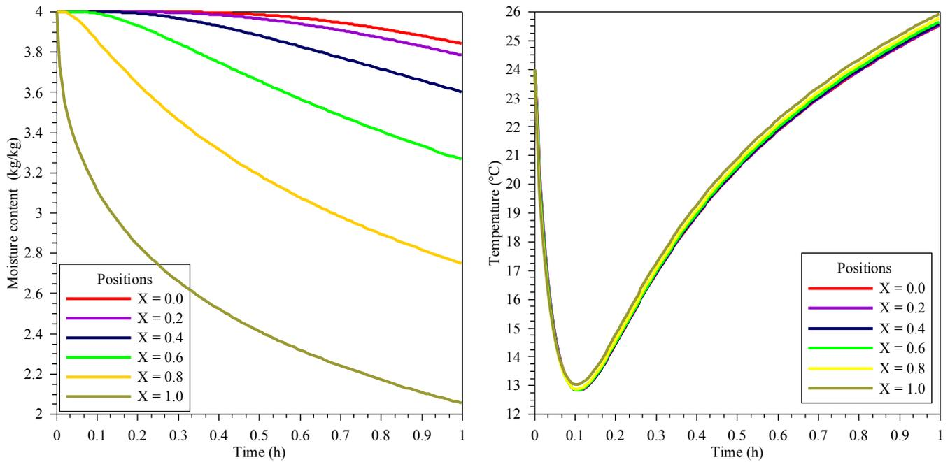
Figure 3. Profiles: (a) moisture content versus time in the first hour of drying, (b) temperature versus time in the first hour of drying
