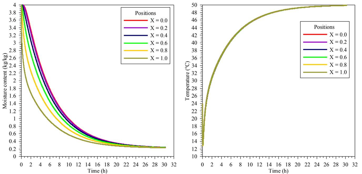
Figure 4. Profiles: (a) moisture content versus time along the whole domain, (b) temperature versus time along the whole domain.
