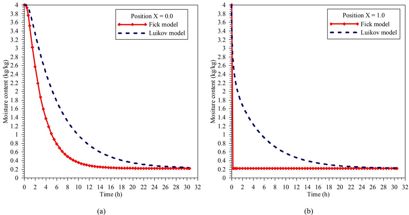
Figure 2. Comparison between the distributions of moisture content with the of Fick and Luikov models.
