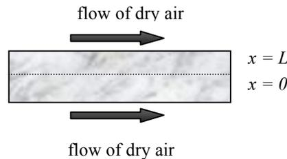
Figure 1. Geometry for the drying of a moist porous medium.
