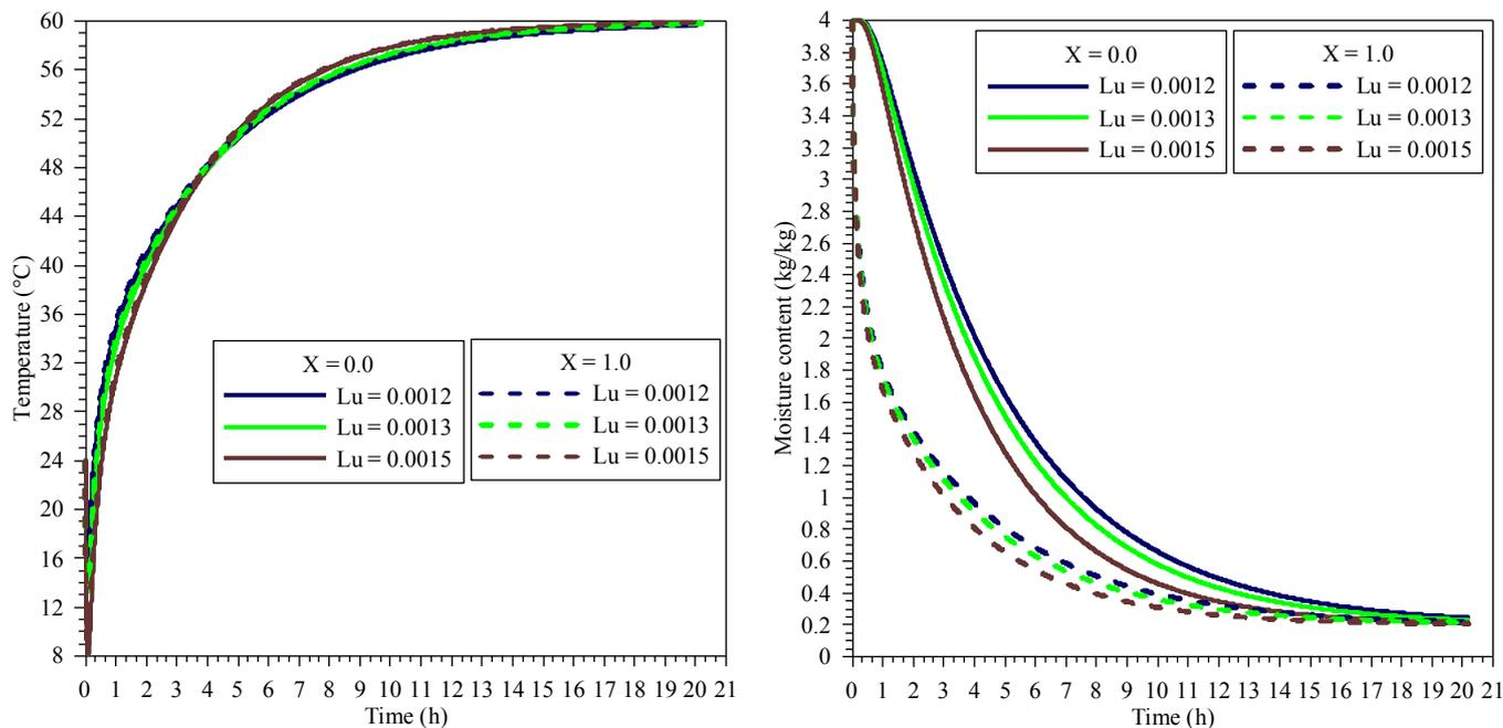
Figure 6. Profiles for the values  $Biq = 0.135$ ,  $Bim = 2.43$ ,  $Pn = 0.142$ ,  $Ko = 74.32$  e  $\varepsilon = 0.3$ , varying  $Lu$ : (a) temperature versus time along the whole domain, (b) moisture content versus time along the whole domain.
