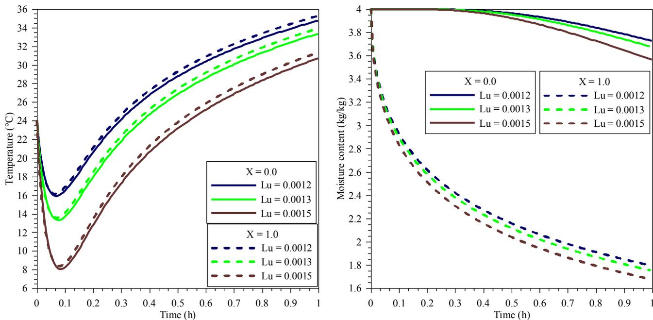
Figure 5. Profiles for the values  $Biq = 0.135$ ,  $Bim = 2.43$ ,  $Pn = 0.142$ ,  $Ko = 74.32$  e  $\varepsilon = 0.3$ , varying  $Lu$ : (a) temperature versus time in the first hour of drying, (b) moisture content versus time in the first hour of drying.
