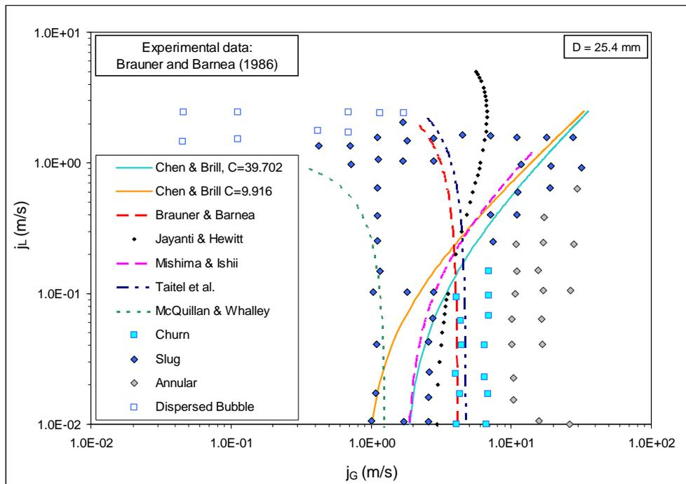
Figure 1. Different theoretical curves for slug-to-churn transition with Brauner and Barnea data (1986) (Air-water, 1.0 bar, 25°C, 25.4 mm ID)
