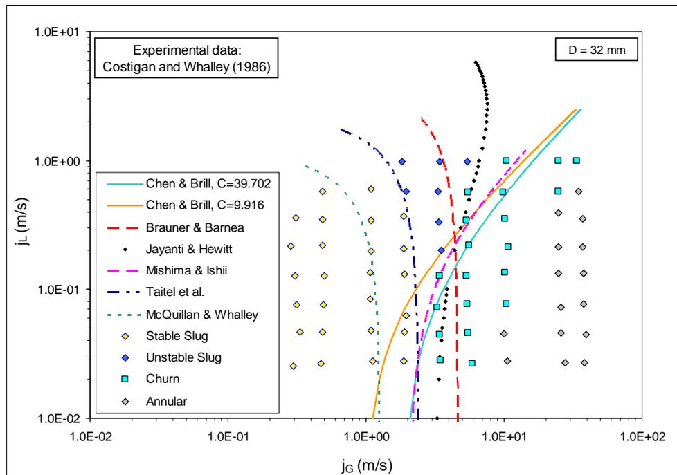
Figure 2. Different theoretical curves for slug-to-churn transition with Costigan and Whalley data (1997) (Air-water, 1.0 bar, 25°C, 32 mm ID)
