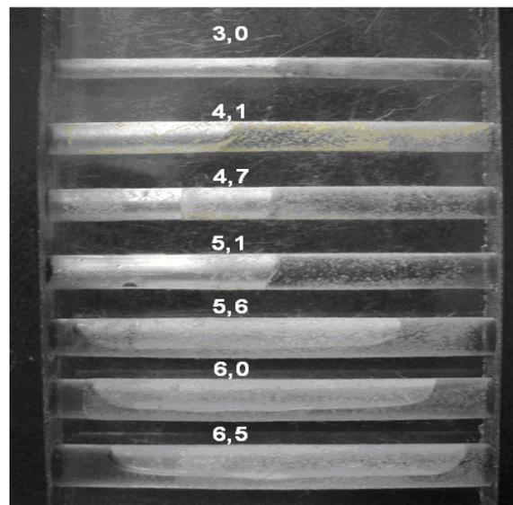
Figure 2. Air-water two-phase flow distribution inside horizontal round channels (diameter in millimeters)
