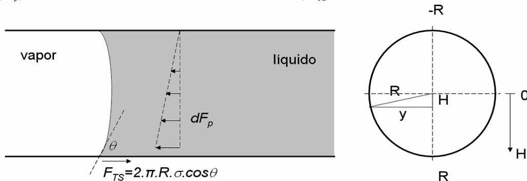
Figure 1. Pressure and surface tension used in the stratified condition model.
